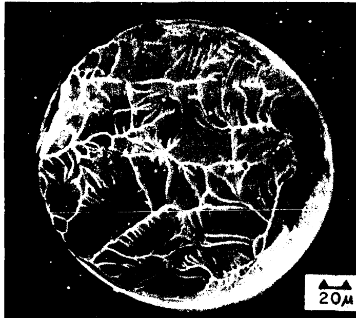
FIGURE 19 Fracture surface of \text{Pd}_{77.5}\text{Cu}_6\text{Si}_{16.5} wire fractured at 1 atm. The fracture surface is inclined at \approx 45^\circ , sloping down from left to right (Davis, 1978).
