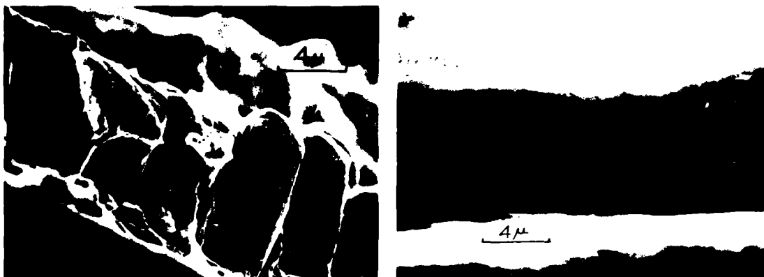
FIGURE 7. ION PLATED COPPER SAMPLES(FRACTURE SECTIONS)
