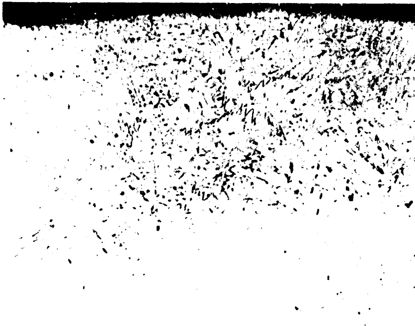
Fig.11 Vanadium carbide alloying of carbon steel (x 500)
