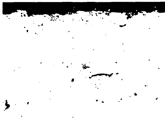
Fig. 16: Transverse micro-section of a copper-coating sprayed in a low-pressure atmosphere, 200 : 1, unetched
