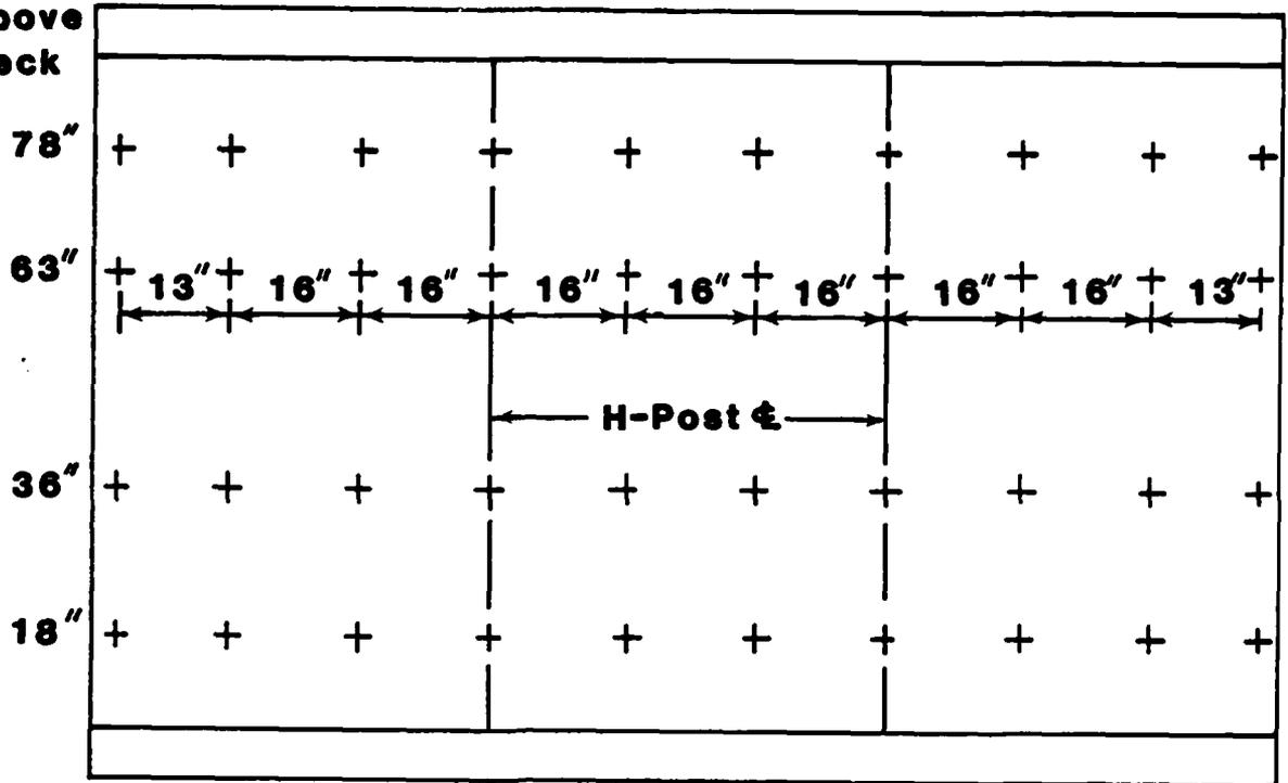
**Instrumentation Compartment Bulkhead**
