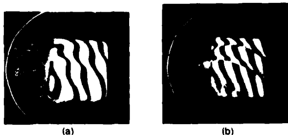
Fig. 8. Interferograms of the OPD of an SLM: (a) 0 V; (b) 5 V, 6 kHz.
