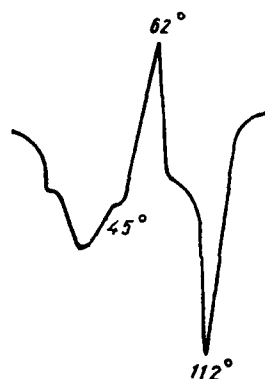
Fig. 49. Thermogram of heating amorphous specimen/sample PU-2.
