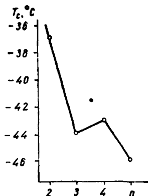
Fig. 17. Dependence T_c on a quantity of \text{CH}_2 -group in the glycol segment of polyurethane chain.
