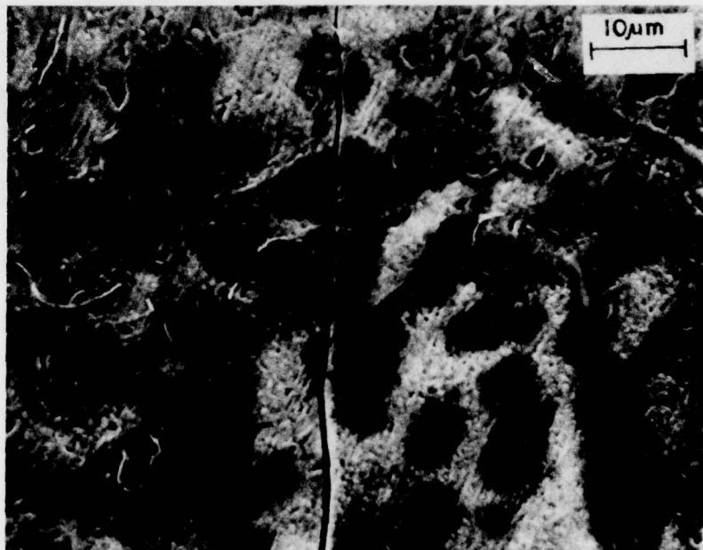
Fig. 11 — Iron particles embedded in silicate platelet on delaminated surface. Higher magnification of Figure 10.
