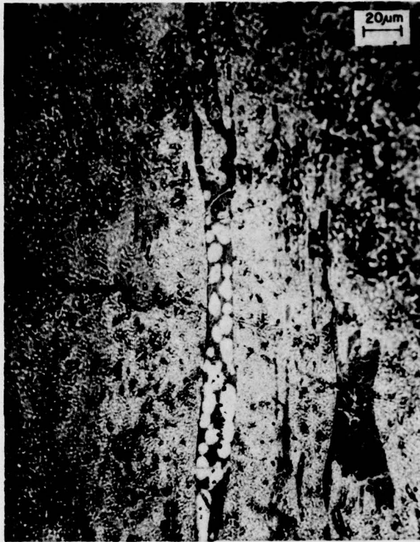
Fig. 3 — Optical micrograph showing two phase silicate particle embedded in rust
