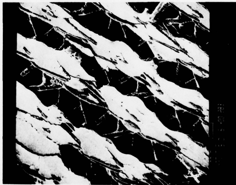
Figure 9. Scanning electron micrographs of matching failure surfaces from a lap shear specimen of Ti6Al4V - FM400 adhesive.
