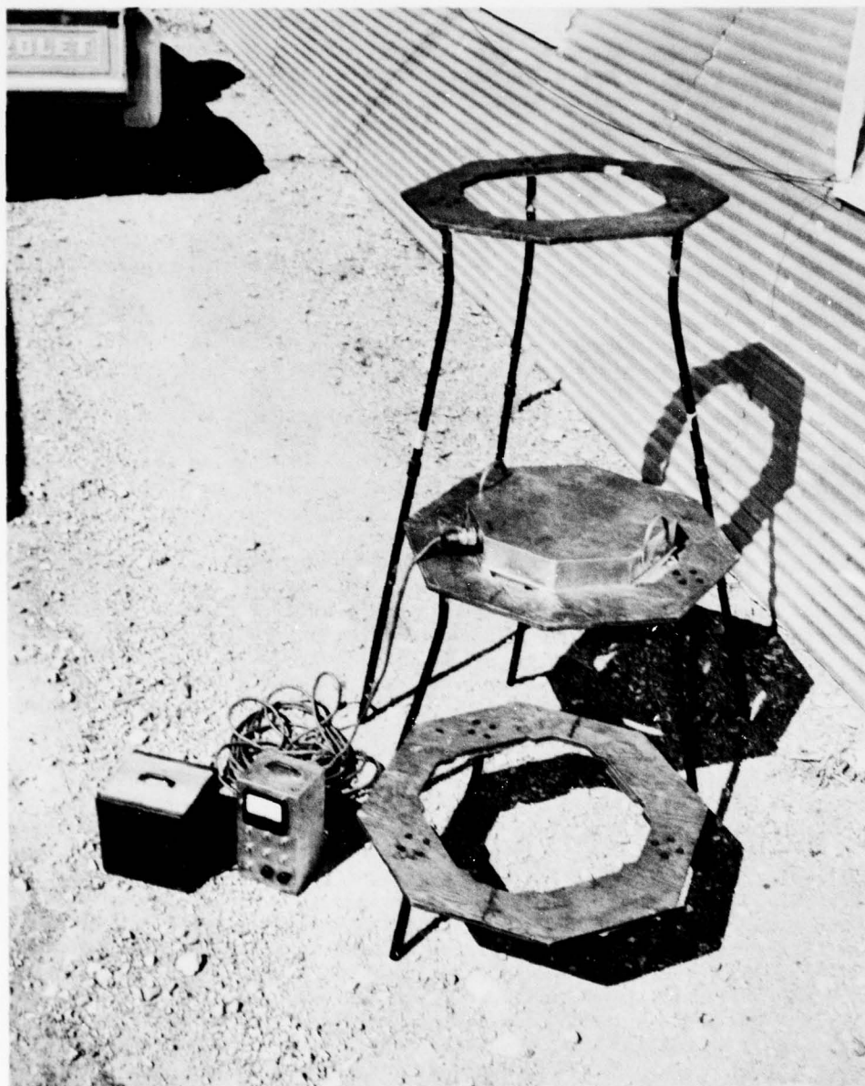
Fig. 2.2--Table mounts for beta-absorption instrument. The instrument can be seen mounted on center table.
