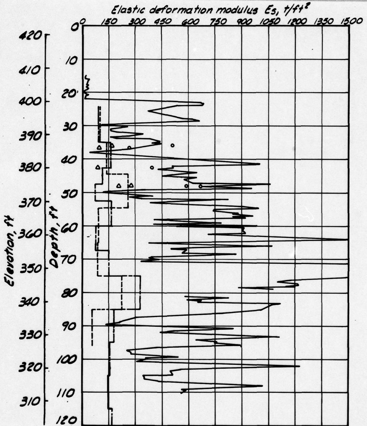
Static cone penetration tests
