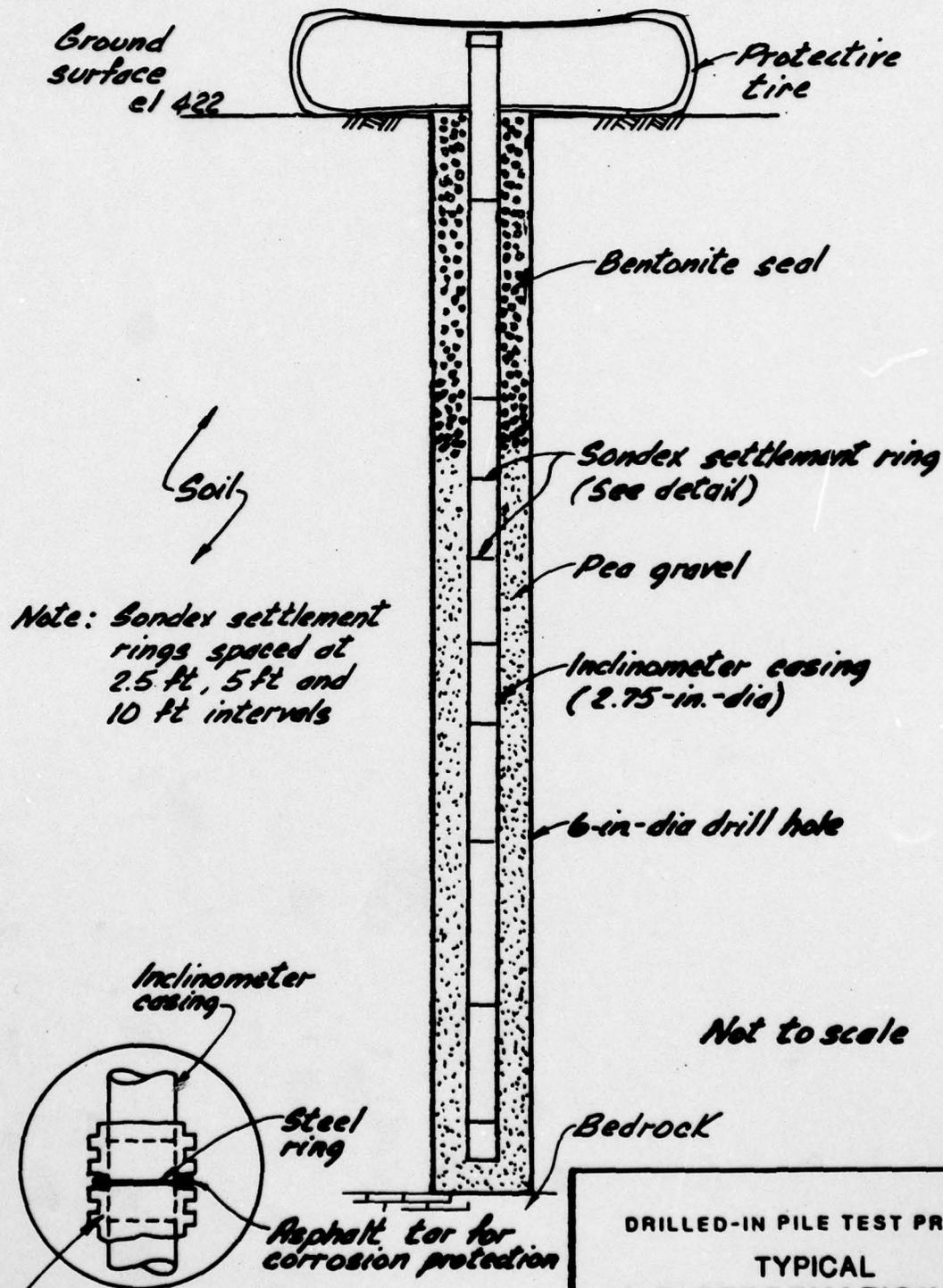
**DRILLED-IN PILE TEST PROGRAM**
