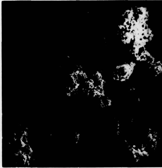
Fig. 1 Agglomerated, molten salt synthesized LZT powder. SEM, 1000X.
