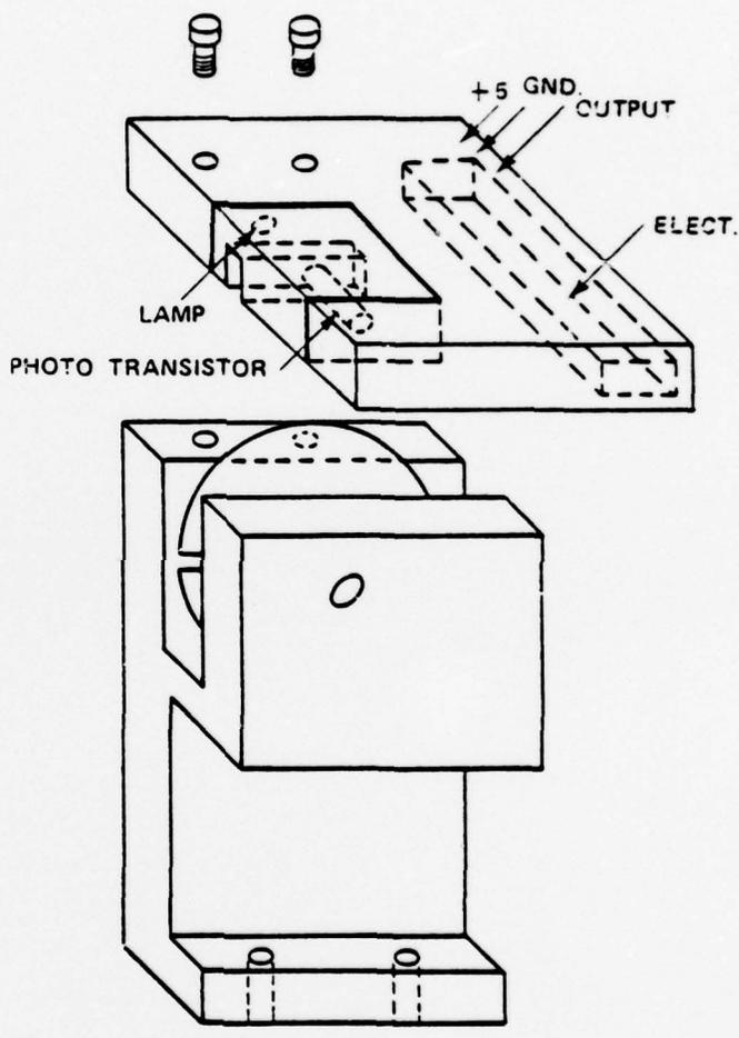
Figure 4: Monochromator Channel Advance
