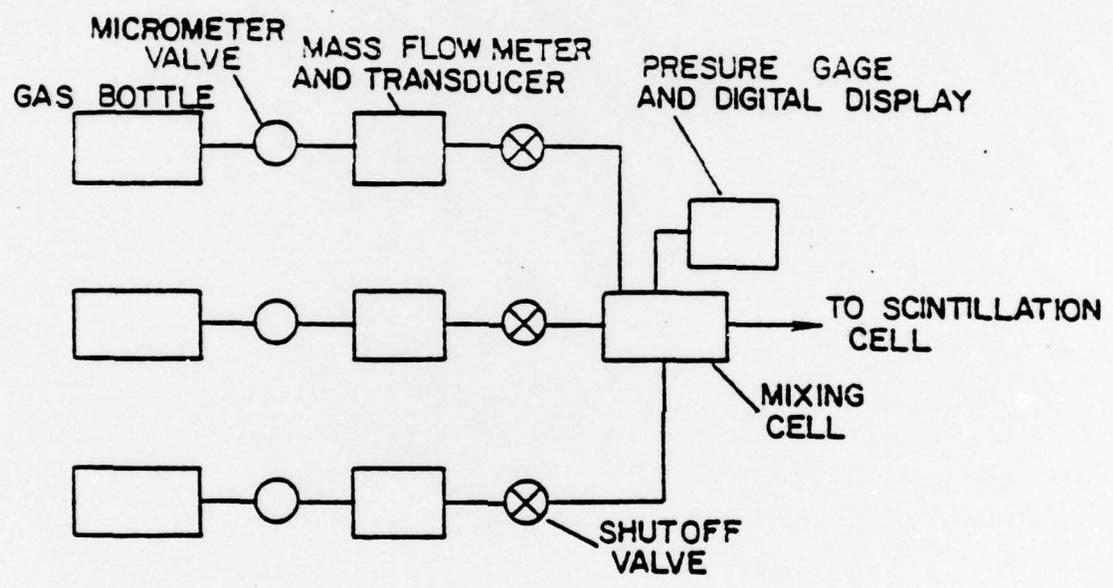
Figure 2 : Gas Handling System
