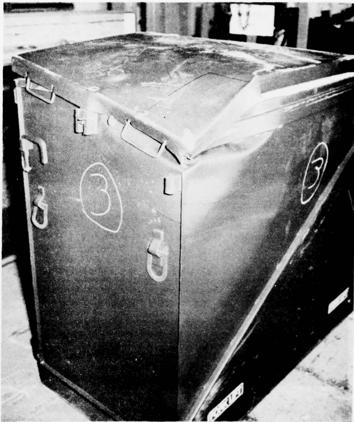
FIGURE 11. DAMAGE FROM FOUR FOOT DROP ON CONTAINER DESIGN C
