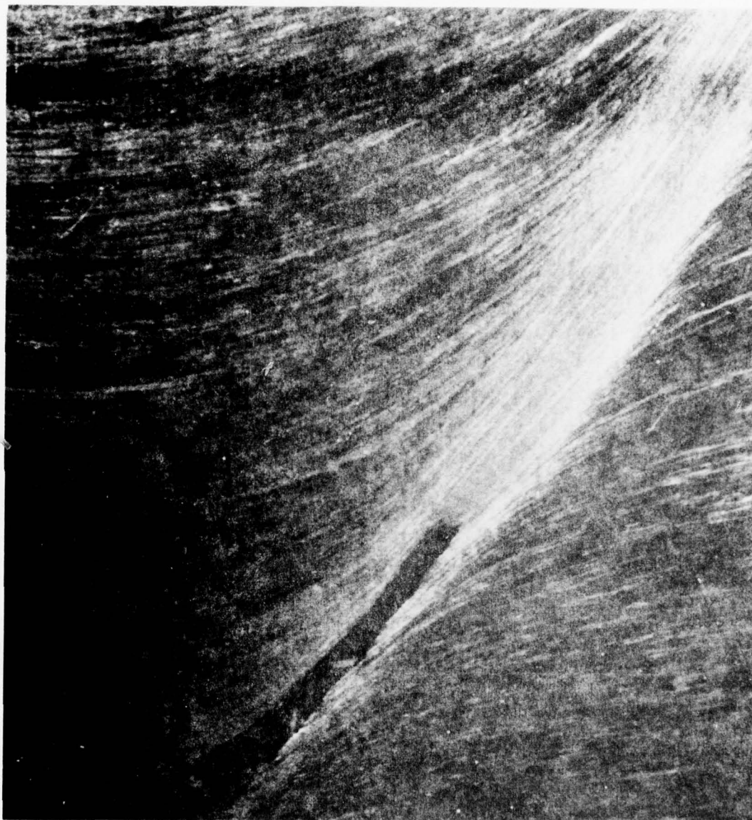
Fig. 6. Propagation of the defect at two-thirds development. Note the blunted tip and sharply defined band of localized shear.
