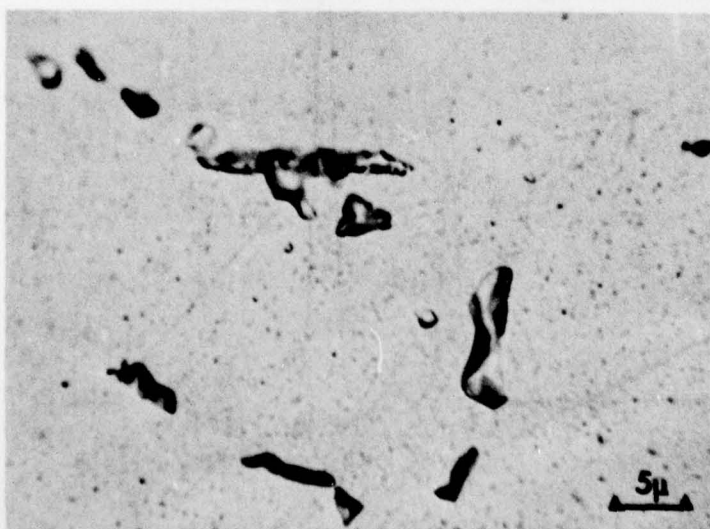
FIG 9 GRAIN BOUNDARY SIGMA PHASE IN 316 ss AGED AT 650°C FOR 22,800h
