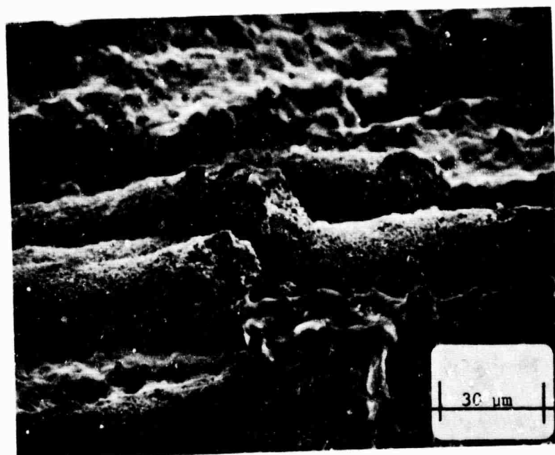
Fig. 6. Fracture surface of \text{Al}_2\text{O}_3 :PZT composite showing degradation of fiber surface in contact with the matrix phase.
