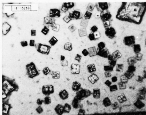
Fig. V-24. An optical micrograph of KCl crystallites grown on a smooth SiO 2 surface. The magnification is 500X.
