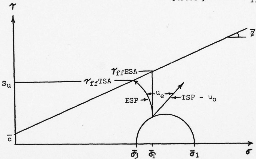
$$\tau_{ffESA} = \bar{c} + \bar{\sigma}_f \text{TAN } \bar{\phi}$$
