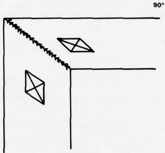
c. Probe contact location for 45° butt welds:
