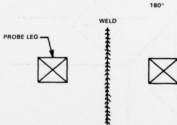
b. Probe contact location for 90° butt welds (location of probes are to be the same on the interior of the welds).
