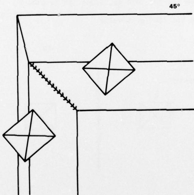
d. Probe location for interior welds of an I-beam or T-beam to a plate:
