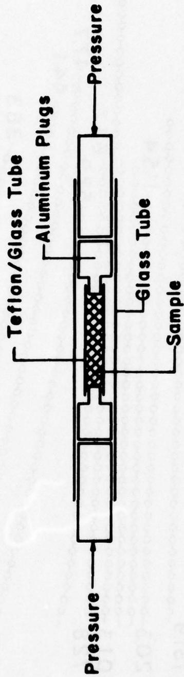
Figure A.1 Setup for the Sample Molding
