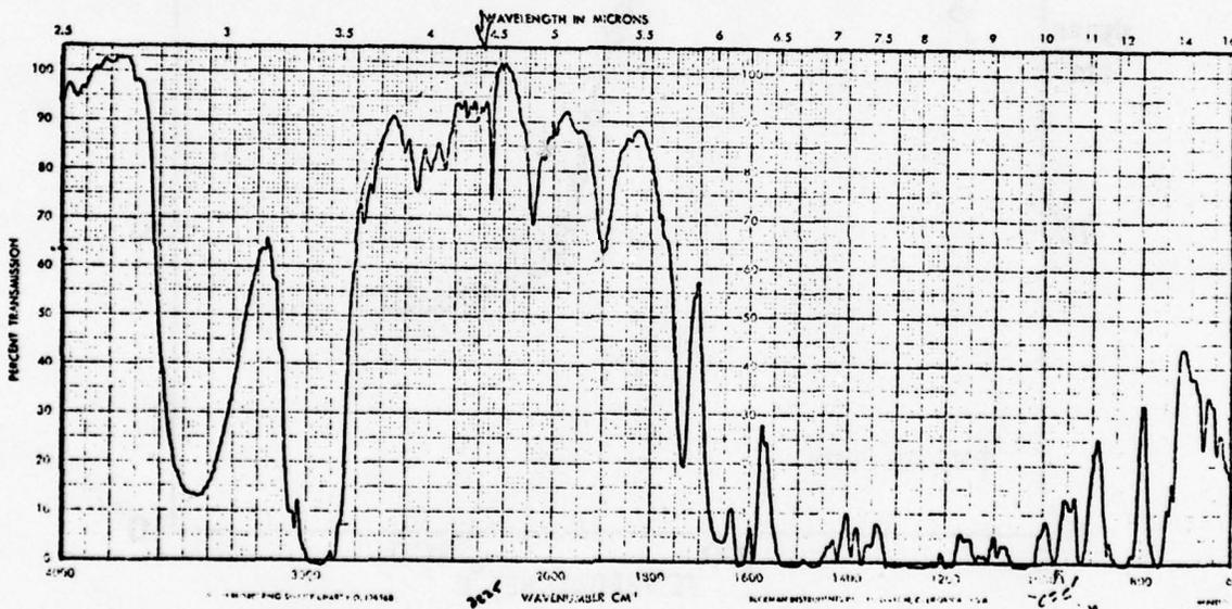
Figure 12 Infra-red Spectrum of RE-A, Extracted Resin
