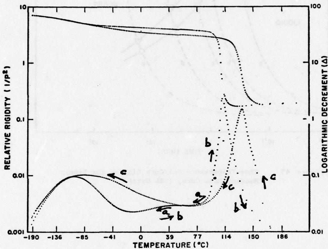
Figure 46 Rigidity and Damping versus Temperature (TBA plot) of Epon 836/5% Curing Agent Cured for 200 Hours at 80°C.
