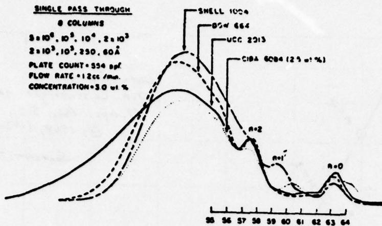
Epoxy resin GPC spectra resulting from one pass through eight columns.
