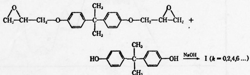
**Figure 1** Molecular Structure of Bisphenol A Diglycidyl Ether (DGEBA) Epoxy Resins.
