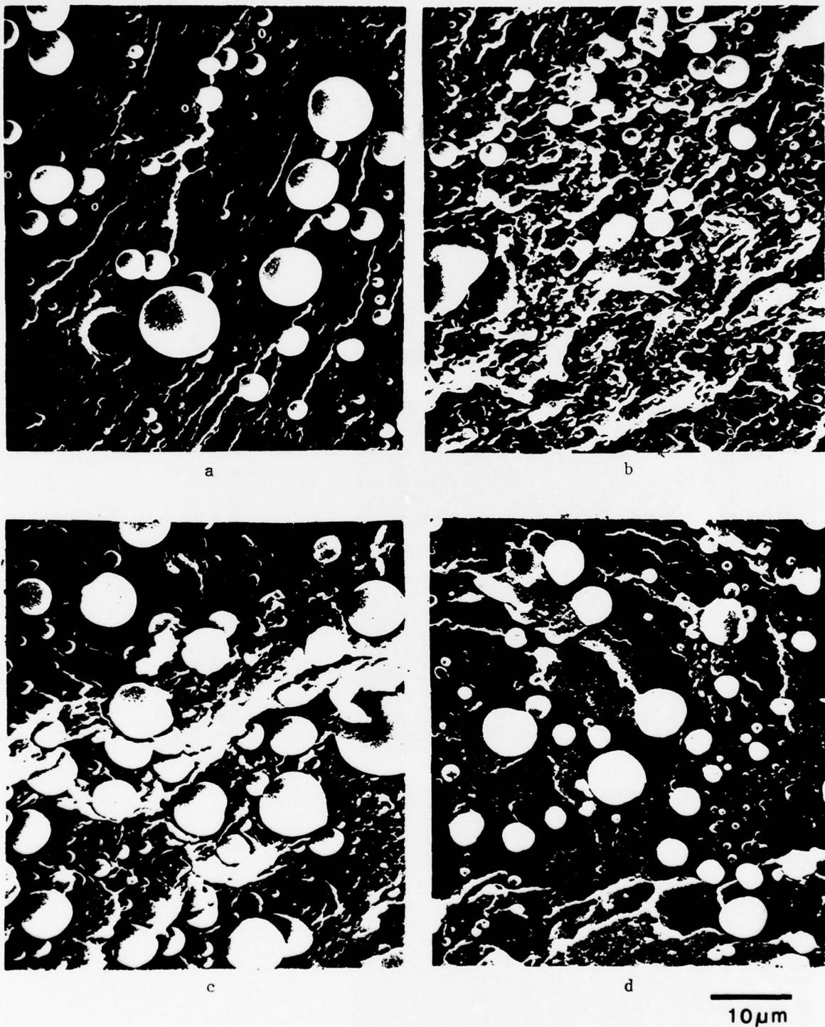
**Figure 33** Scanning Electron Micrographs of Fracture Surfaces of RE-A Neat Resin Cured at (a) 75°C for 30 Hours (b) 120°C for 2 Hours (c) 150°C for 2 Hours (d) 165°C for 2 Hours. Cured Specimens Fractured After Cooling in Liquid Nitrogen
