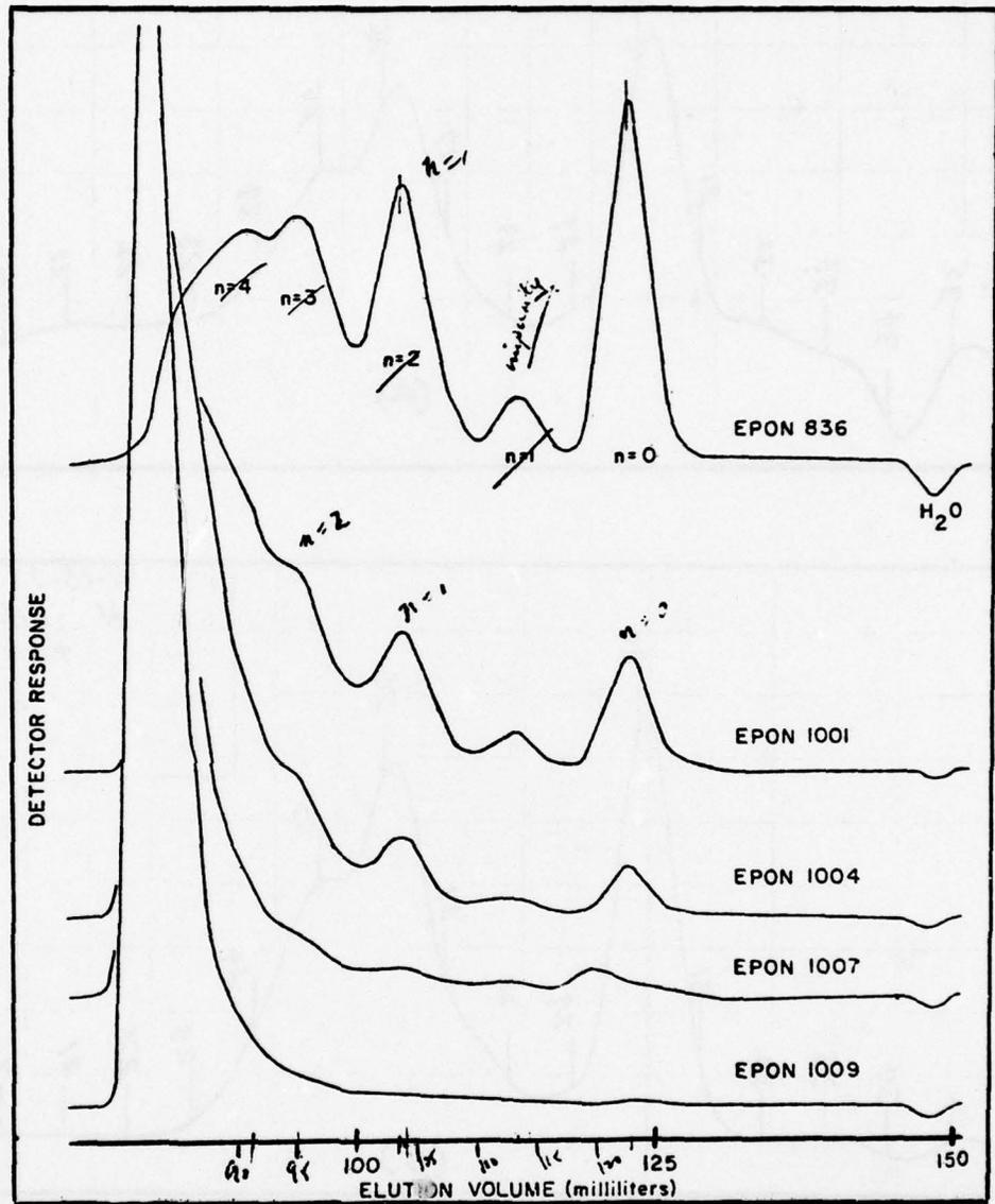
Figure 17 Gel Permeation Chromatograms of Epoxy Resins.
