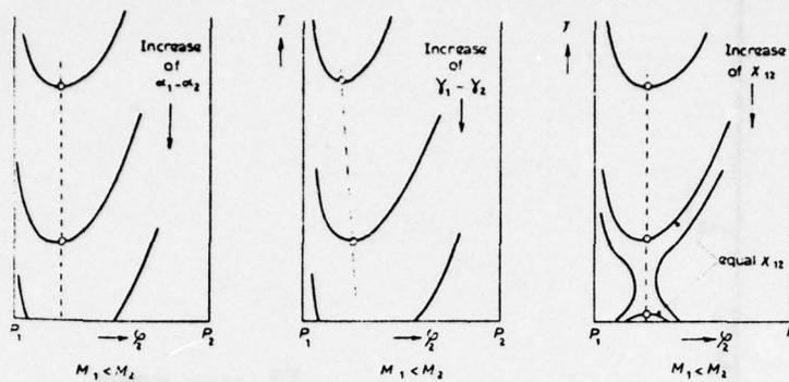
**Figure 39** Computed Dependence of Miscibility Gap in Two-Polymer Mixtures on Equation of State Parameters (a)  $\alpha$  = Thermal Expansion Coefficient, (b)  $\gamma$  = Thermal Pressure Coefficient, (c) Interaction Energy Parameter,  $X_{12}$ . (From McMaster ref. 21)
