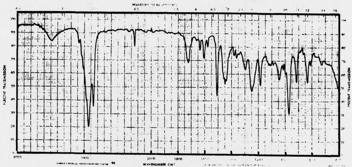
**Figure 21**      **Infra-red Spectrum of the High Molecular Weight Fraction Separated by GPC (see Figure 20)**
