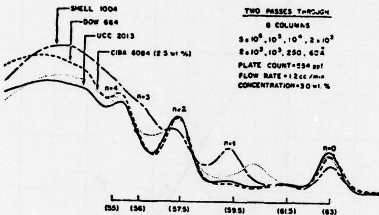
Epoxy resin GPC spectra resulting from two passes through eight columns.
