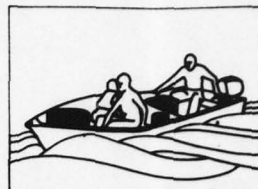
Overloading your boat will reduce its freeboard.
