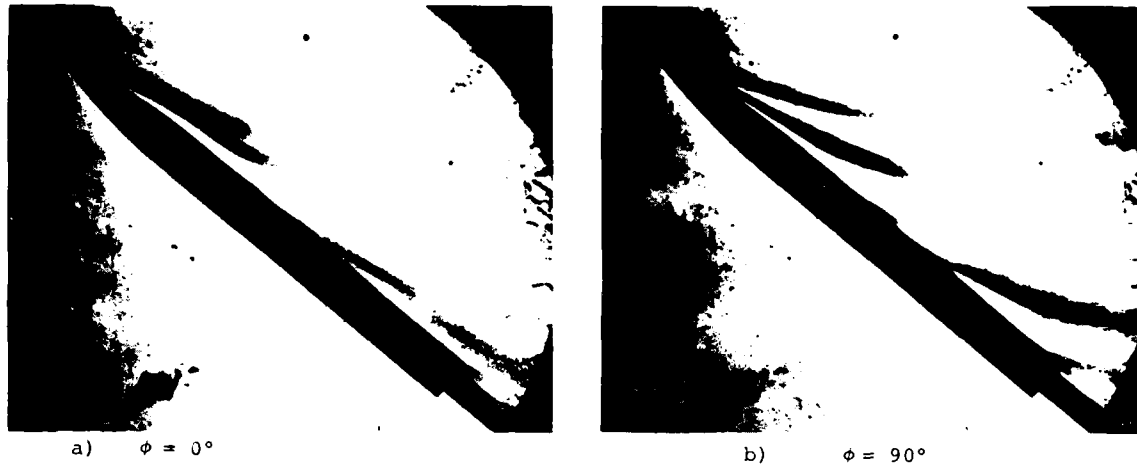
Figure 15. Variation of the leeward flowfield with changes in roll orientation on an axisymmetric model, M = .7 , \alpha = 40^\circ .
