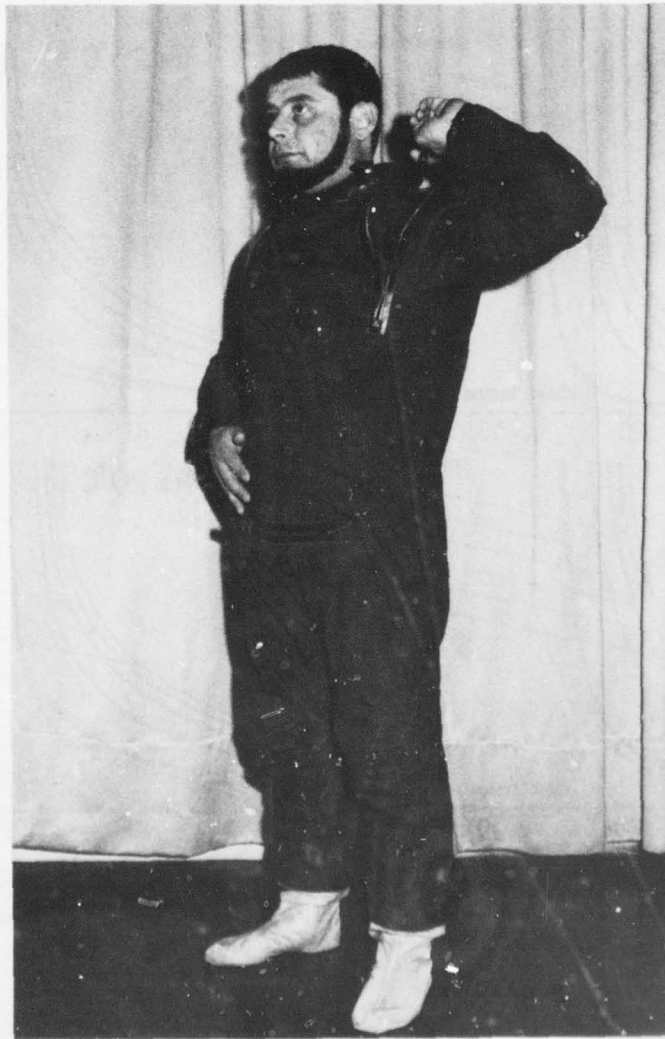
Fig.4.11 Subject wearing the SIA 10.2 suit. Note the position of the zip fastener around his neck, enabling the subject to put it on without assistance
