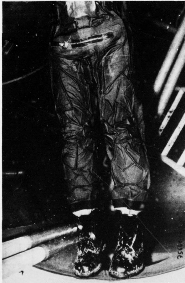
Fig.4.4 Test in water of the SIA 10.2 anti-immersion suit, showing the patchwork pattern on the lower limbs and the abdomen
