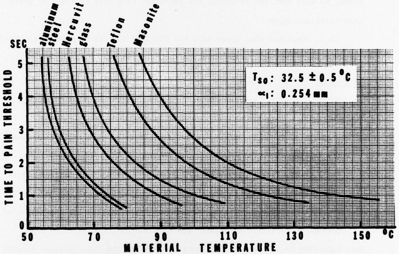
FIGURE 7 - Variations in time to pain threshold at given temperatures due to differences in thermal properties of materials.
