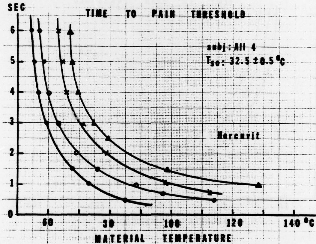
FIGURE 5 - Pain threshold time vs material temperature, ring finger of four subjects, one material.
