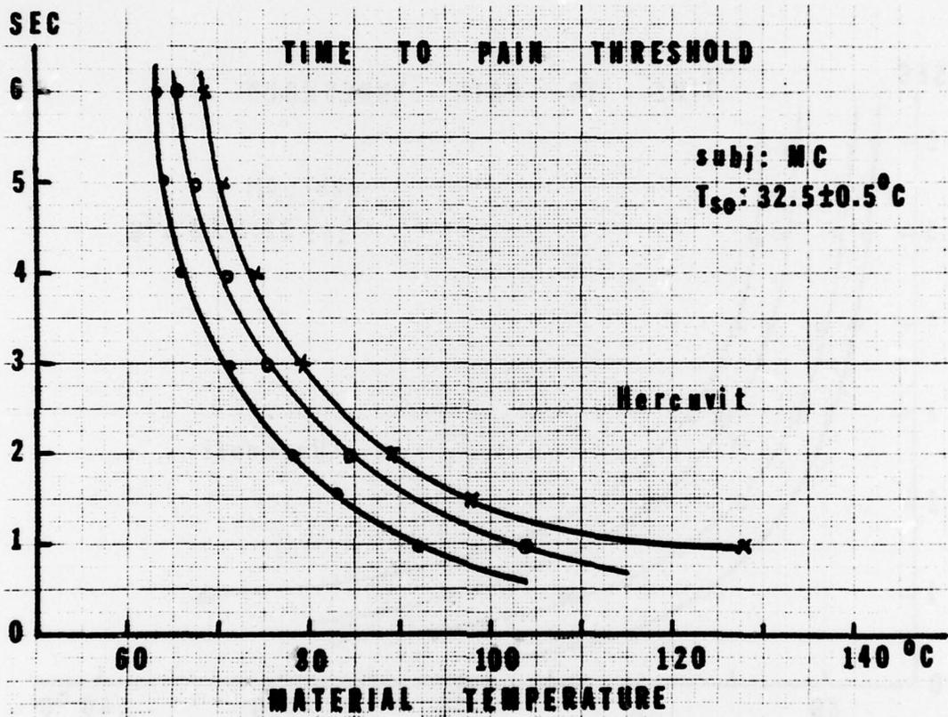
FIGURE 4 - Pain threshold time vs material temperature, three fingers of same hand, one material.
