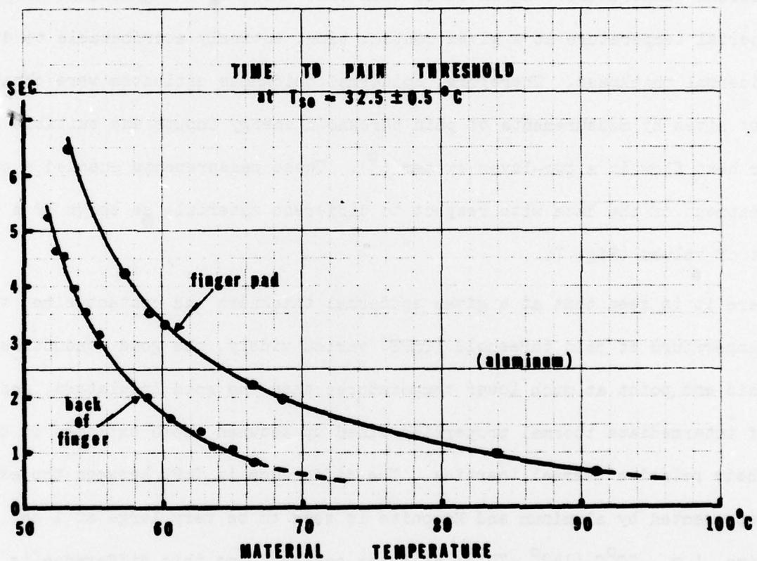
FIGURE 6 - Pain threshold time vs material temperature finger pad and back of same finger, one material.
