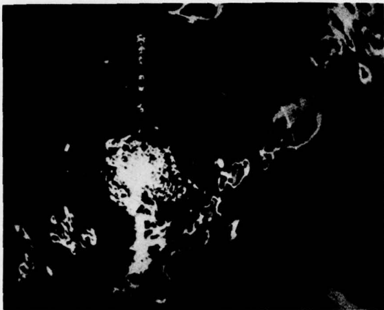
Figure 2-8 WSR-57 weather radar scope presentation for 1733 CST June 12, 1977. Radar contours at approximately 10 dBZ intervals. Range marks (circles) are at 40 km intervals.
