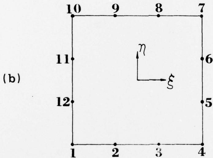
FIGURE 1. (a) 12-NODE CUBIC ELEMENT COLLAPSED TO FORM A SINGULAR ELEMENT;
