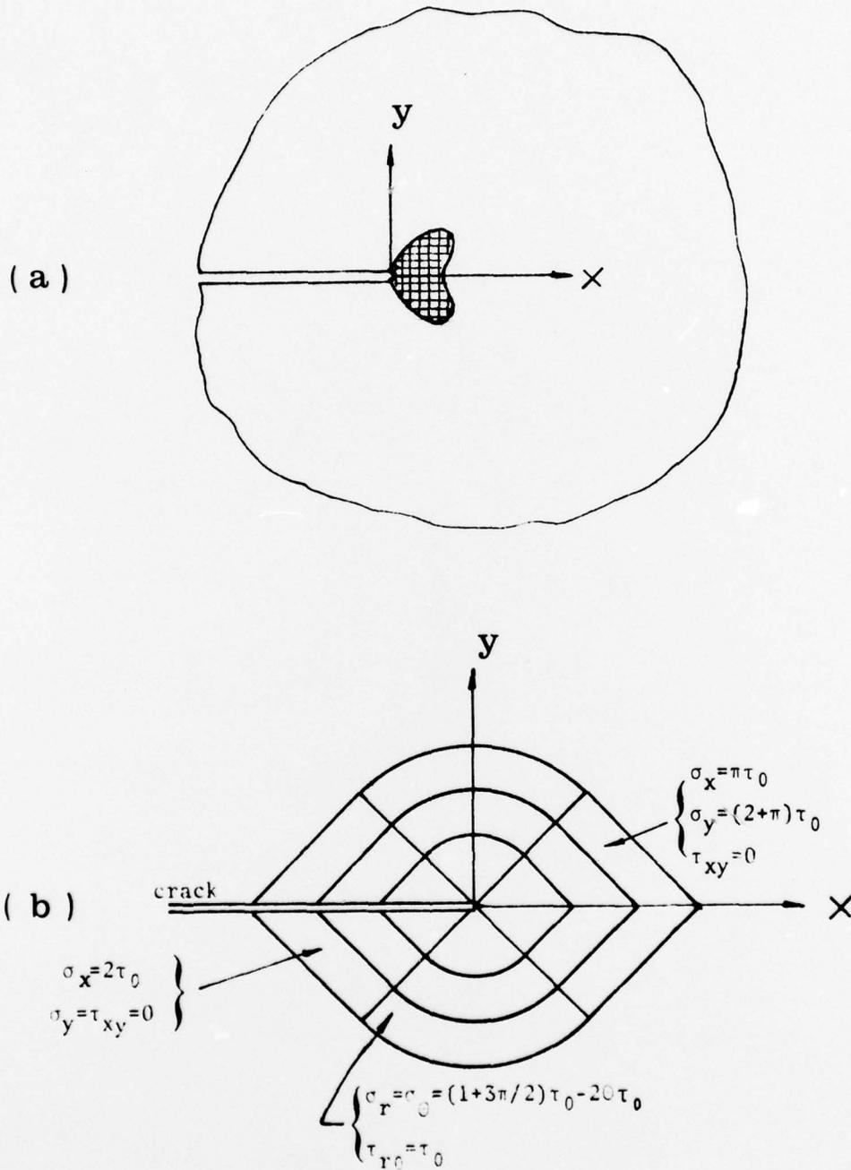
FIGURE 2. (a) SMALL-SCALE YIELDING NEAR A SEMI-INFINITE CRACK;
