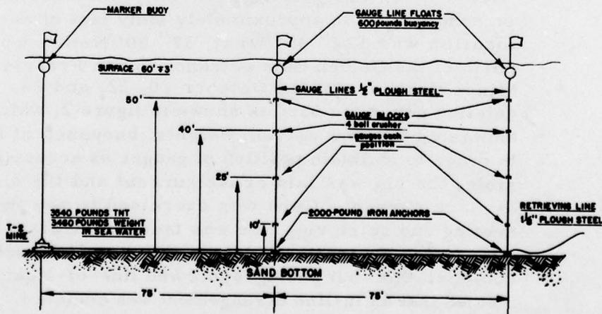
Figure 2. Experimental setup for crusher gauge measurements.
