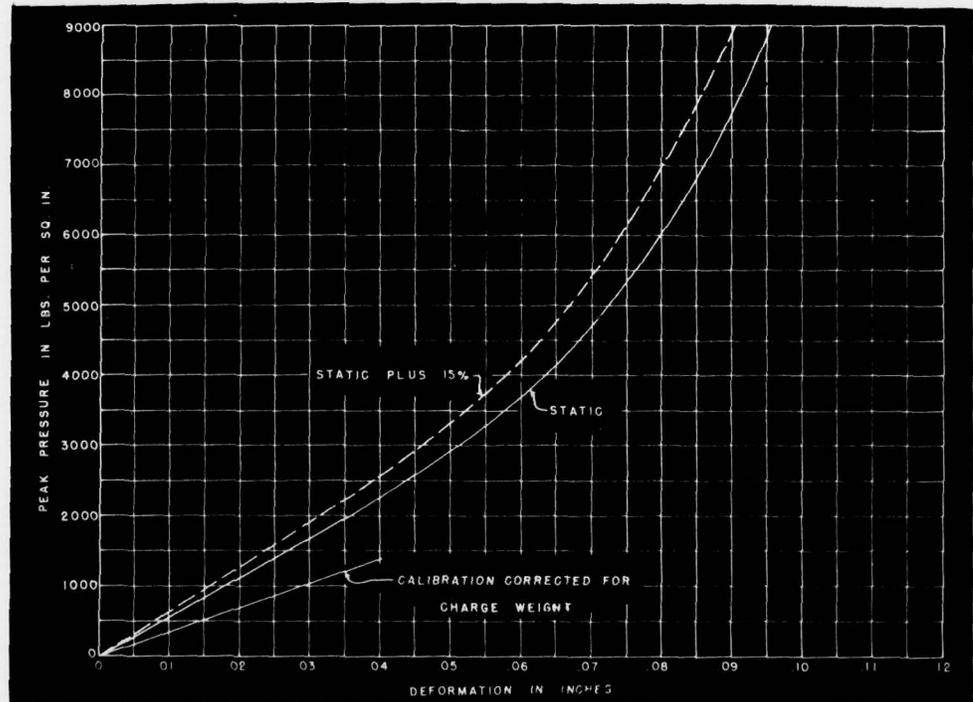
Figure 8. Calibration curves for 5/32-inch copper balls.
