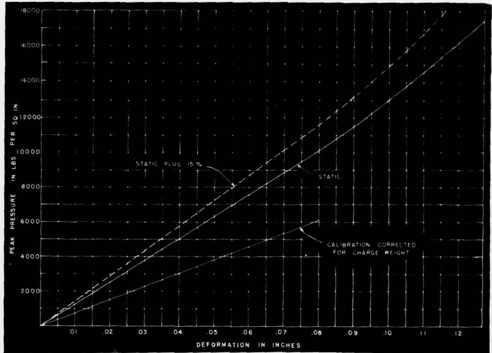
Figure 7. Calibration curves for 3/8-inch copper balls.
