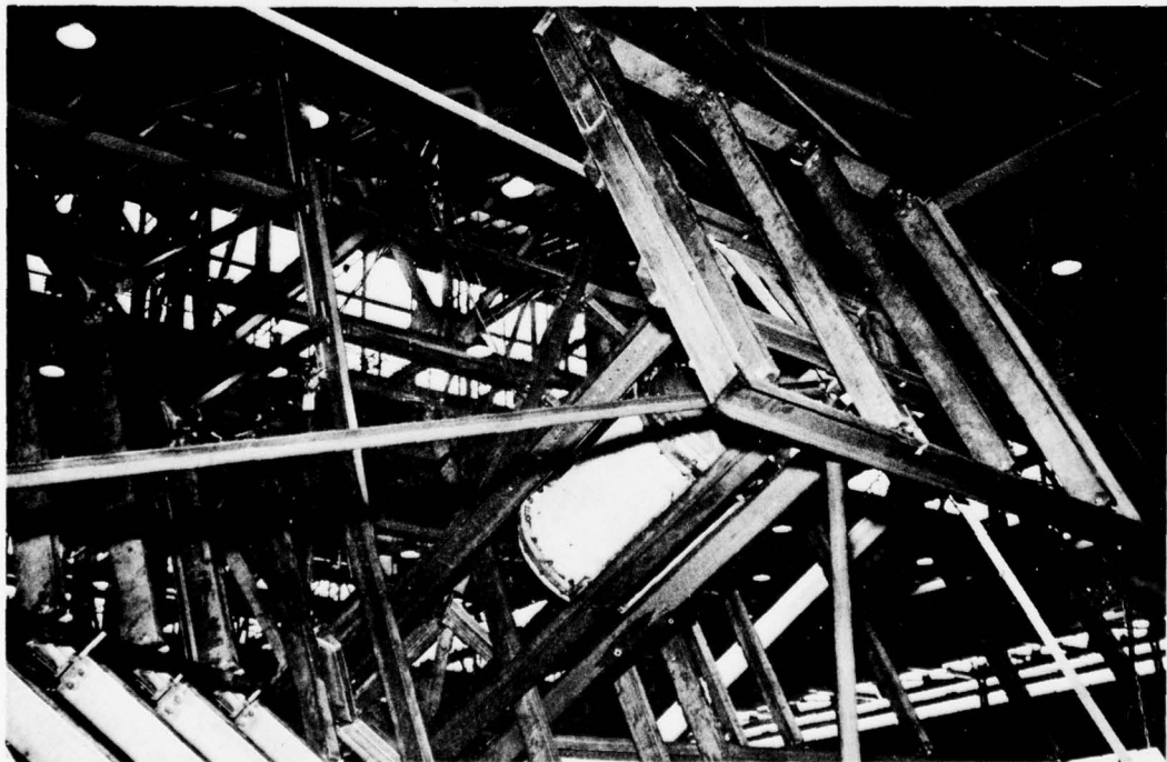
Figure 3. Close-up View of Transducer in the Parabolic Reflector
