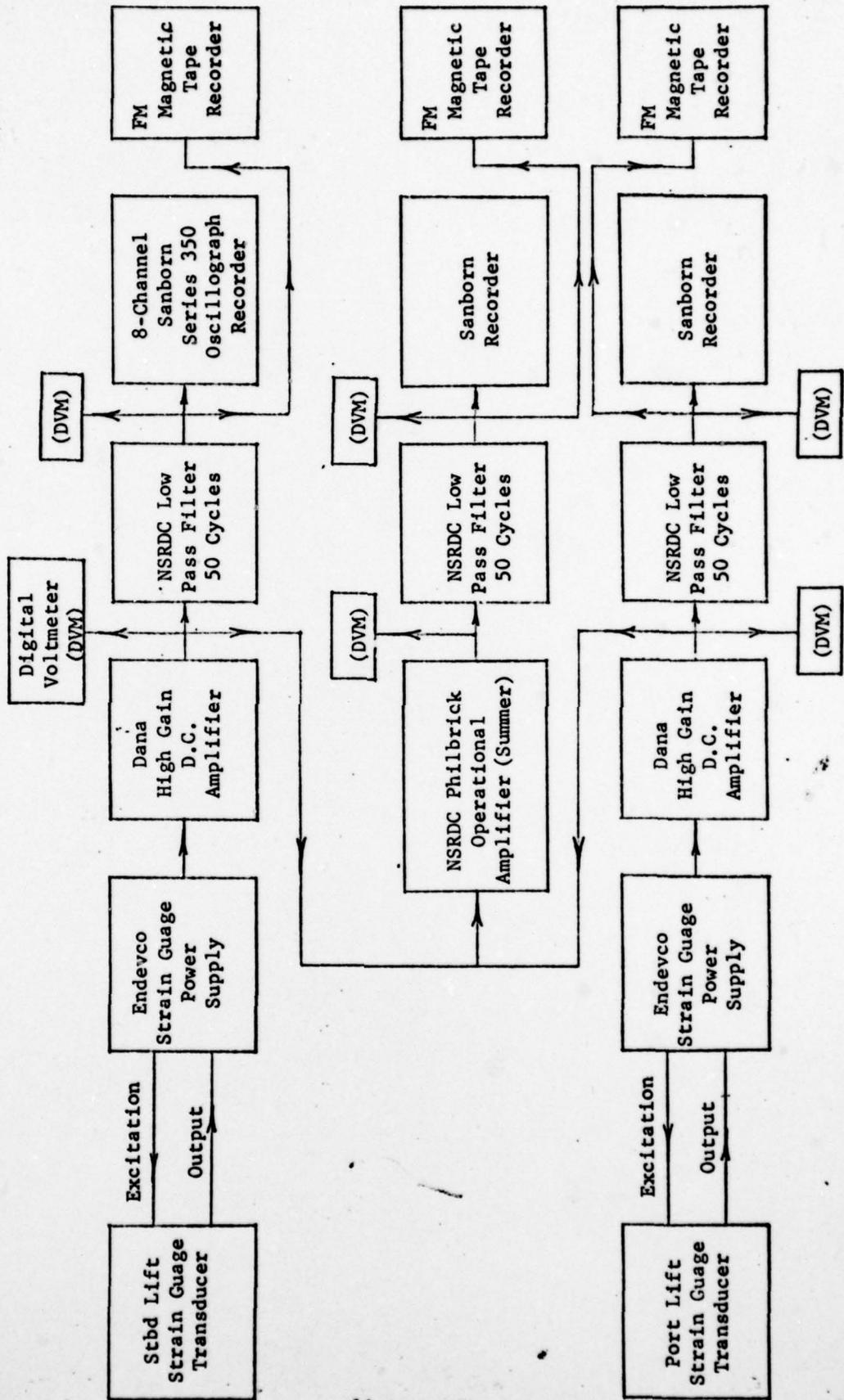
Figure 2 - Block Diagram of Electronic Instrumentation
