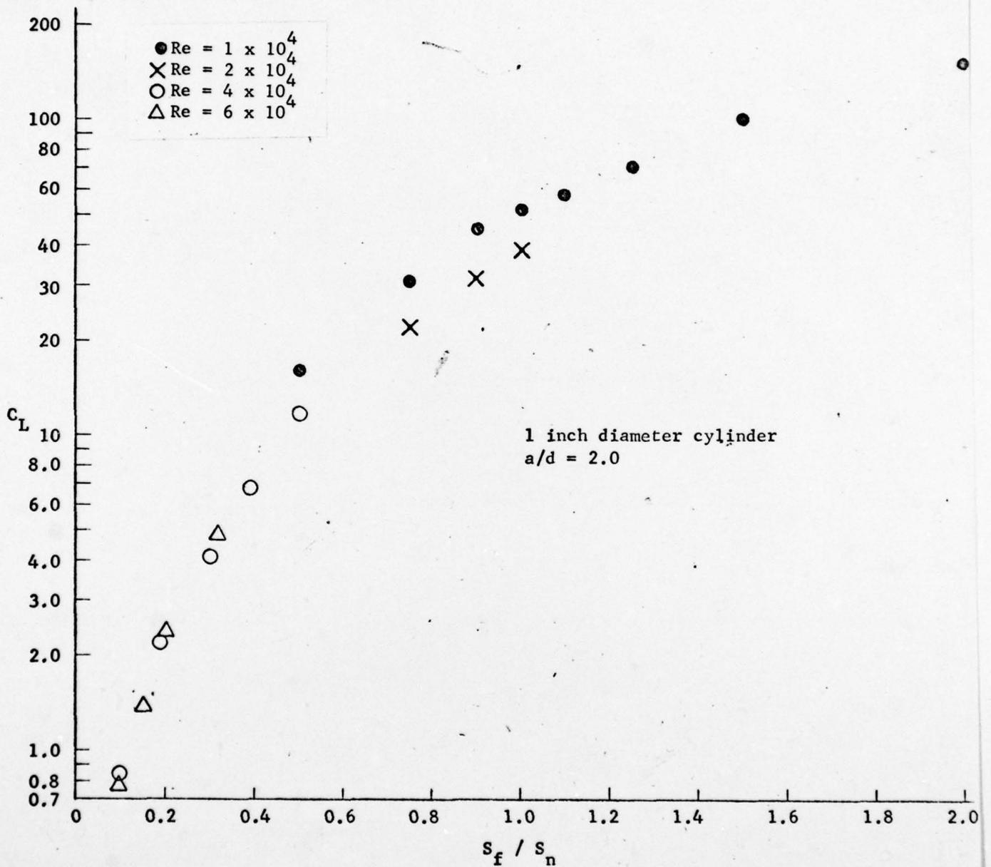
Figure 5 continued - Variation of Lift Coefficient as Function of the Ratio of Forced to Natural Strouhal Numbers for Various Reynolds Number and Ratio of Amplitude to Diameter
