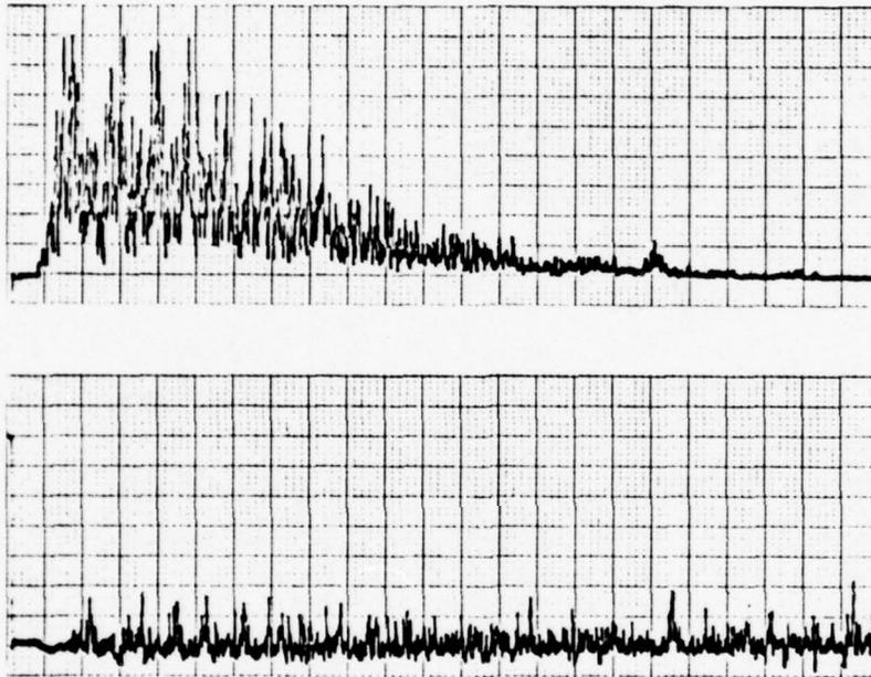
FIG. 3-4 - THE OUTPUT OF A LINEAR CORRELATOR WITHOUT AGC BEFORE AND AFTER NORMALIZATION
