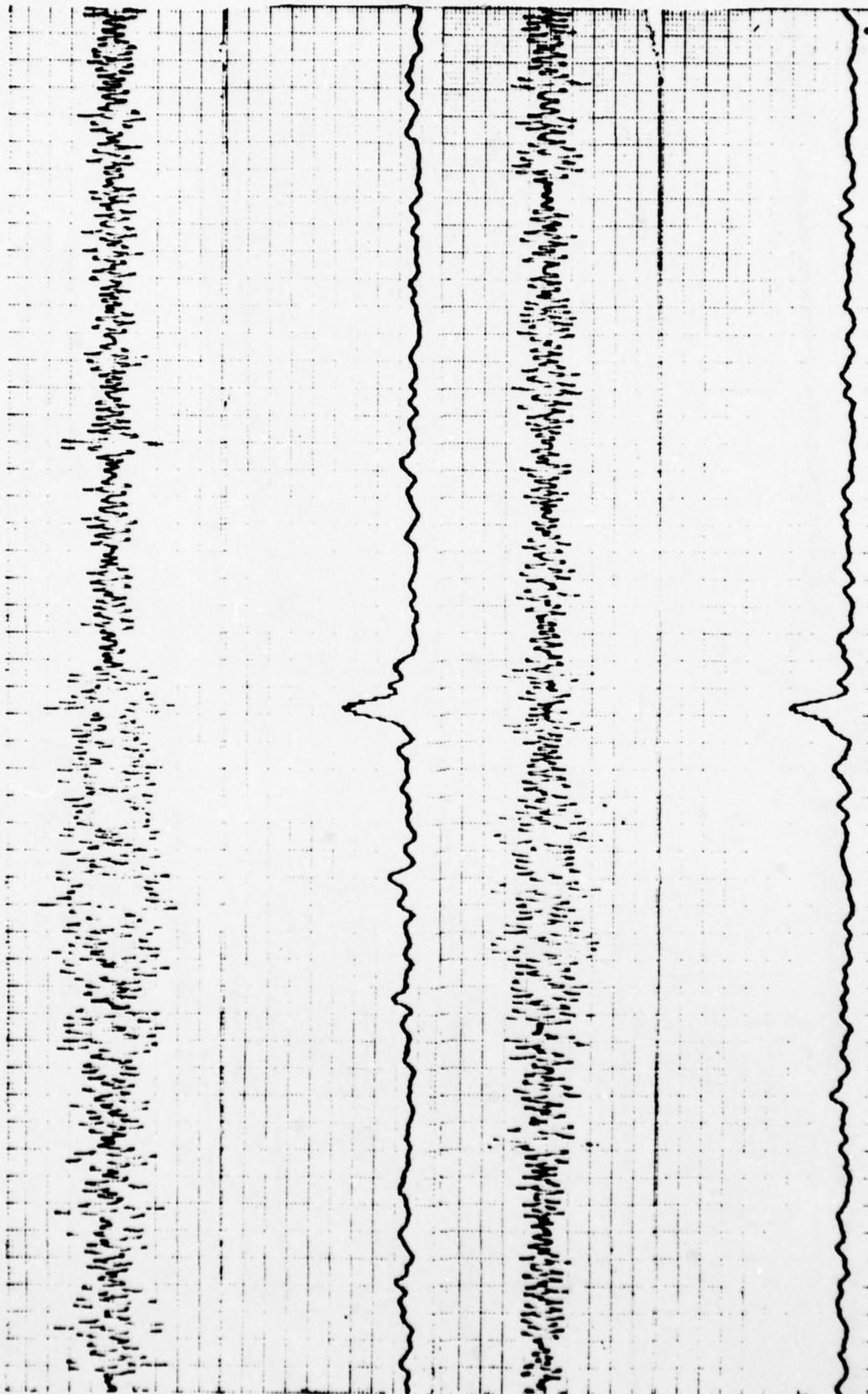
FIG. 2-2 TWO TYPICAL ECHOES FROM THE AN/SQS-26.
