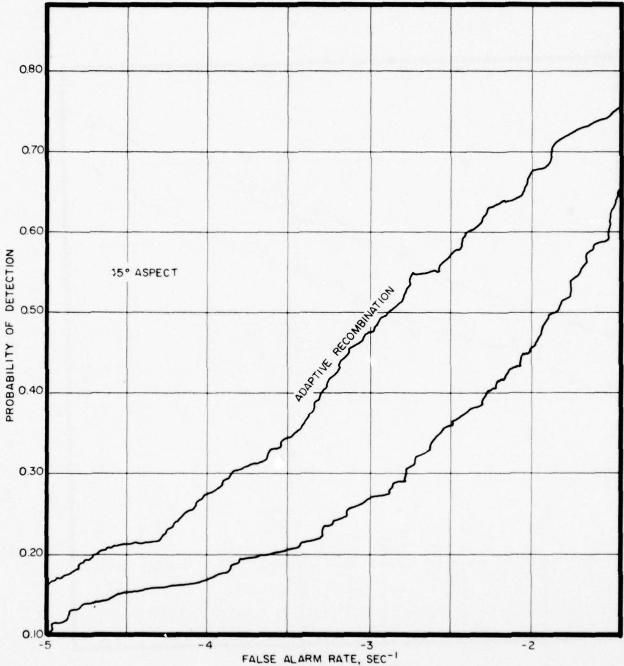
FIG. 2-38 - ADAPTIVE RECOMBINATION COMPARED TO STANDARD LINEAR CORRELATION FOR SEA DATA WITH TARGET AT 45° ASPECT
