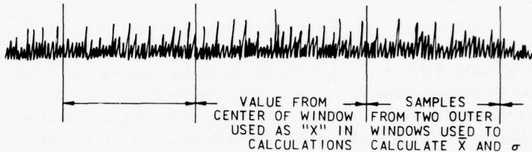
FIG.3-2 - FIRST METHOD OF OBTAINING MEAN AND STANDARD DEVIATION
