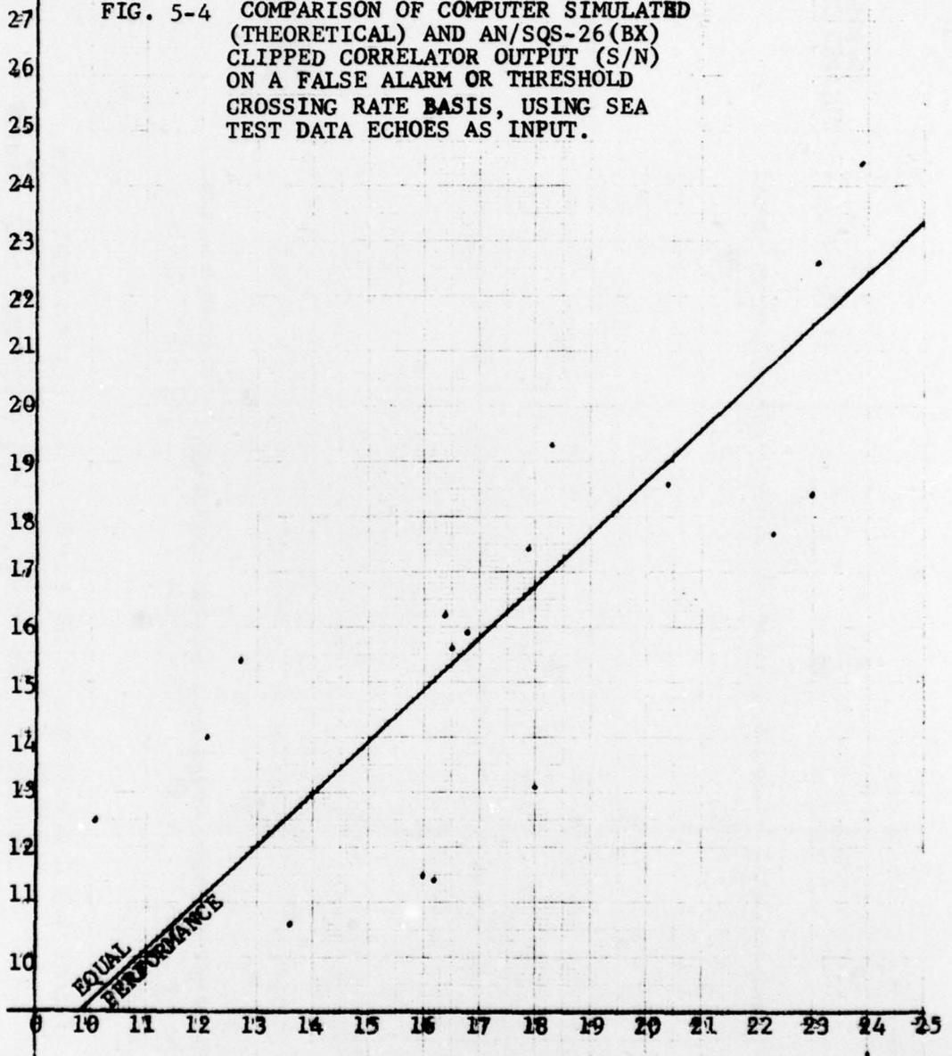
OUTPUT SIGNAL-TO-NOISE RATIO, dB
