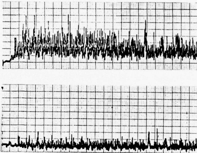
FIG.3-5 - THE OUTPUT OF A LINEAR CORRELATOR WITH AGC BEFORE AND AFTER NORMALIZATION
