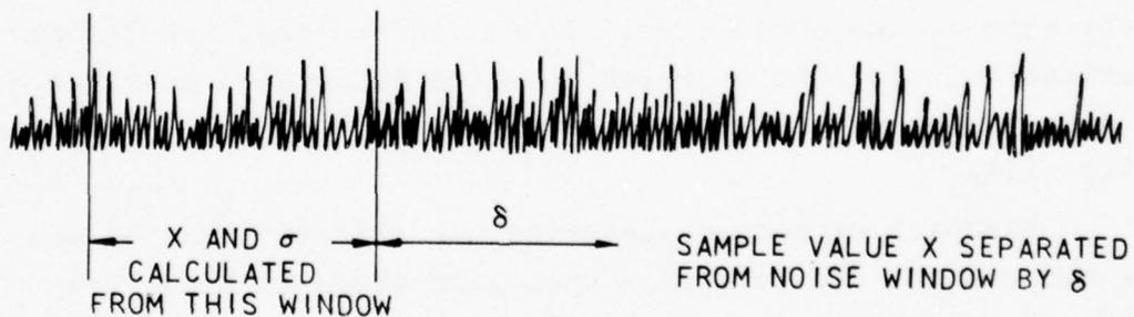
FIG.3-3 - SECOND METHOD OF OBTAINING MEAN AND STANDARD DEVIATION
