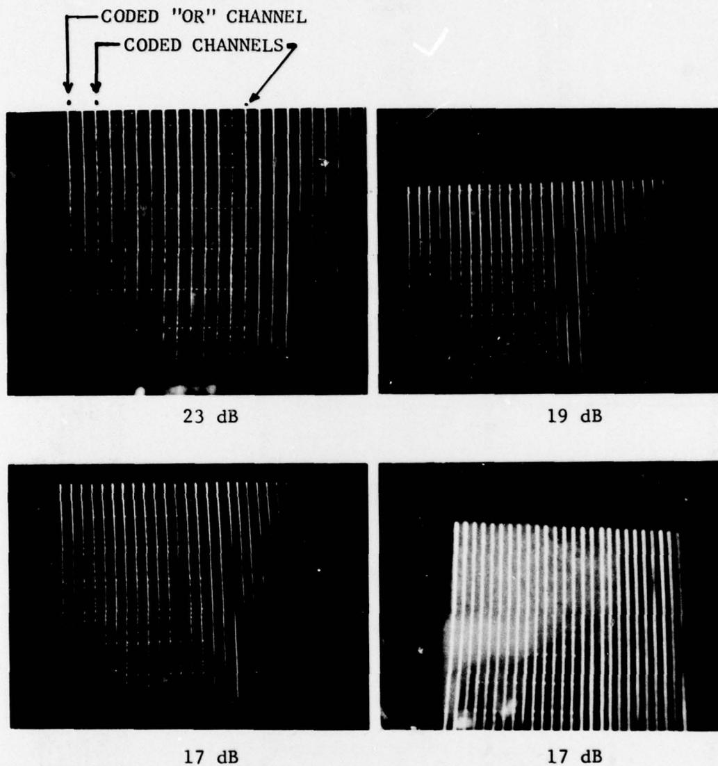
Figure 5-7 PHOTOGRAPHS OF THE AN/SQS-26(BX) DISPLAY USING THE SAME COMPUTER GENERATED INPUTS OF KNOWN AVERAGE INPUT (S/N) TO EACH CODED PROCESSOR CHANNEL. NOMINAL PROCESSOR OUTPUT (S/N) IS INDICATED FOR EACH DISPLAY. TOTAL DISPLAY SWEEP IS 20 SECONDS WITH SIGNALS 3 SECONDS APART.
