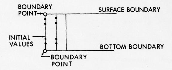
Our methods require the initial conditions and two boundary points before we can proceed to find the solution at the next range line. With this input information, we can classify the boundary descriptions for three different cases, and discuss the treatment of each case separately.
