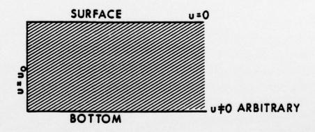
CASE 3: PLANE PARALLEL CONDITIONS WITH UN = 0 AT THE BOTTOM
