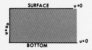
CASE 2: PLANE PARALLEL CONDITIONS WITH u ≠ 0, ARBITRARY AT THE BOTTOM
