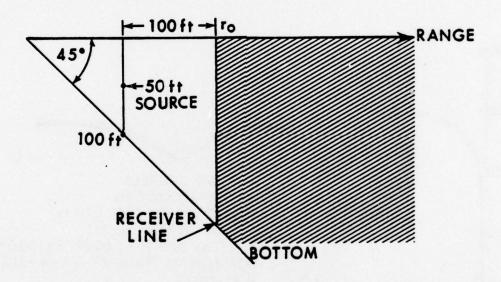
A point source is placed 50 ft below the surface, and the receiver is located 100 ft from the source. The depth of the wedge at the source is 100 ft, the frequency equals 80 Hz, and co equals 5000 ft/sec. The exact solution above indicates the solution of the acoustic wave equation. We attempt to find the parabolic equation solution u in the shaded region, and then we attempt to compare H<sub>0</sub>(1)(kr)u against the acoustic wave equation solution computed by the WEDGE program.
