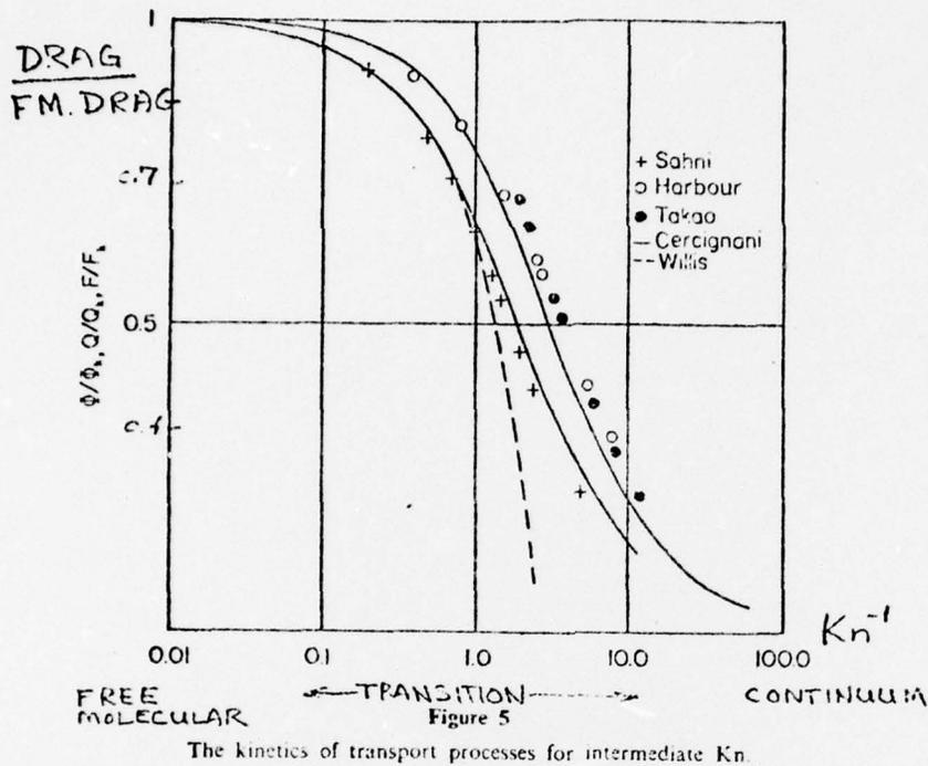
Figure 1. Particle Drag at Low Pressures
