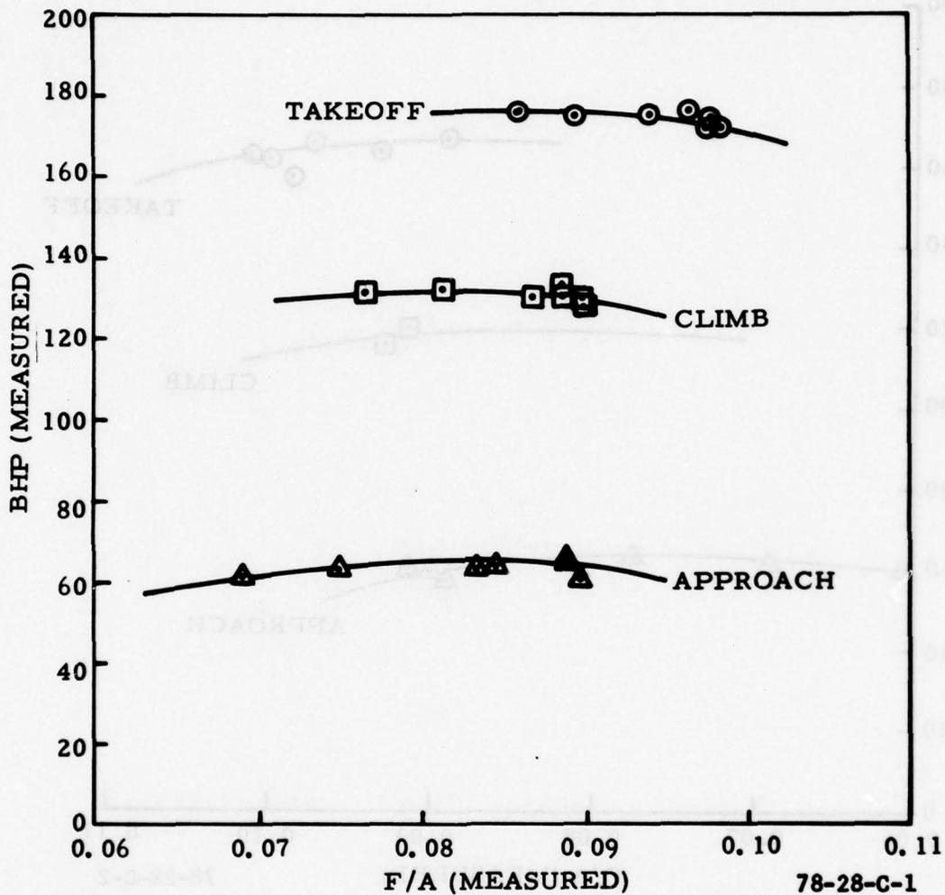
FIGURE C-1. MEASURED PERFORMANCE--AVCO LYCOMING IO-360-B1BD ENGINE--TAKEOFF, CLIMB, AND APPROACH MODES--NOMINAL SEA LEVEL AIR DENSITY 0.0777 lb/ft<sup>3</sup>
