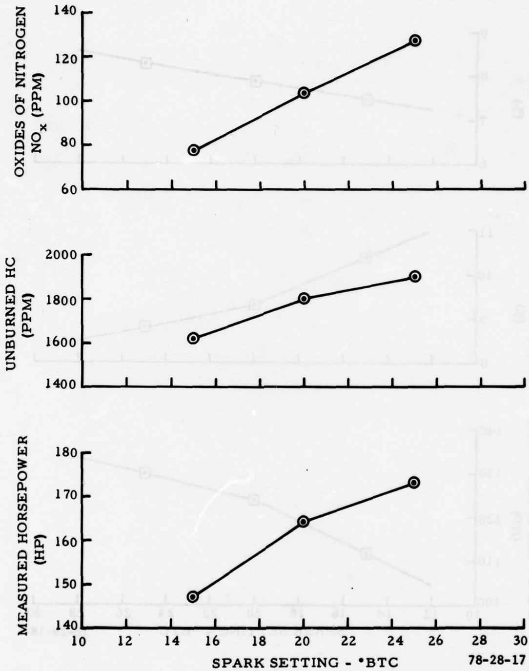
FIGURE 17. EFFECT OF VARYING SPARK SETTING ON ENGINE PERFORMANCE EXHAUST EMISSIONS--TAKEOFF MODE (HC AND NO<sub>x</sub>)
