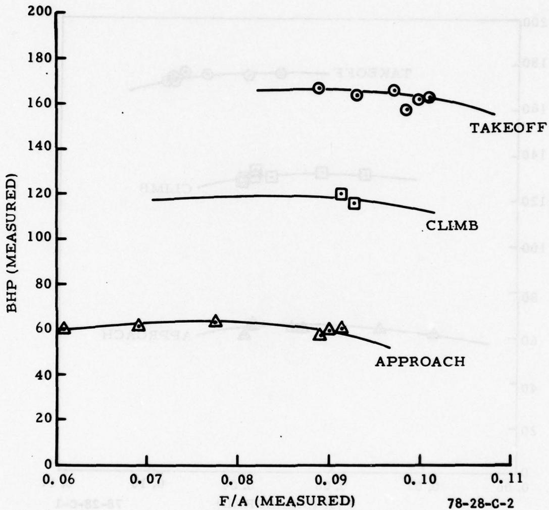
FIGURE C-2. MEASURED PERFORMANCE--AVCO LYCOMING IO-360-B1BD ENGINE--TAKEOFF, CLIMB, AND APPROACH MODES--NOMINAL SEA LEVEL AIR DENSITY 0.0720 lb/ft<sup>3</sup>
