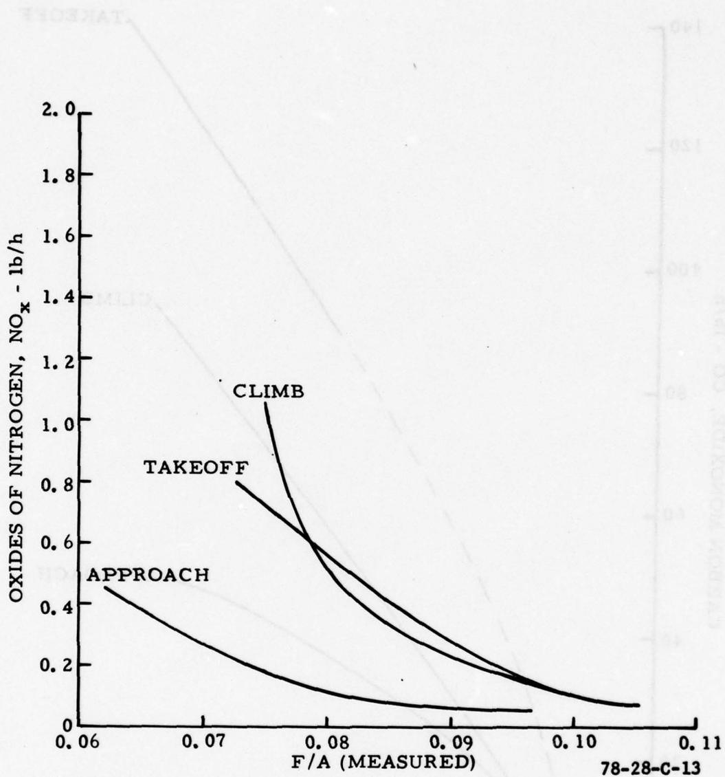
FIGURE C-15. SEA LEVEL STANDARD-DAY EMISSION CHARACTERISTICS FOR AN AVCO LYCOMING IO-360-B1BD ENGINE—OXIDES OF NITROGEN
