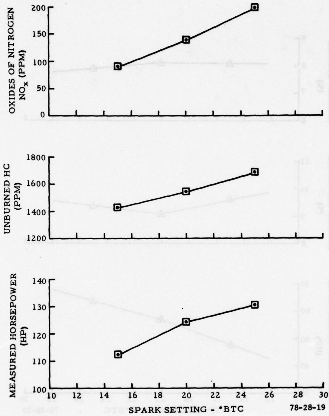
FIGURE 19. EFFECT OF VARYING SPARK SETTING ON ENGINE PERFORMANCE AND EXHAUST EMISSIONS—CLIMB MODE (HC AND NO<sub>x</sub>)
