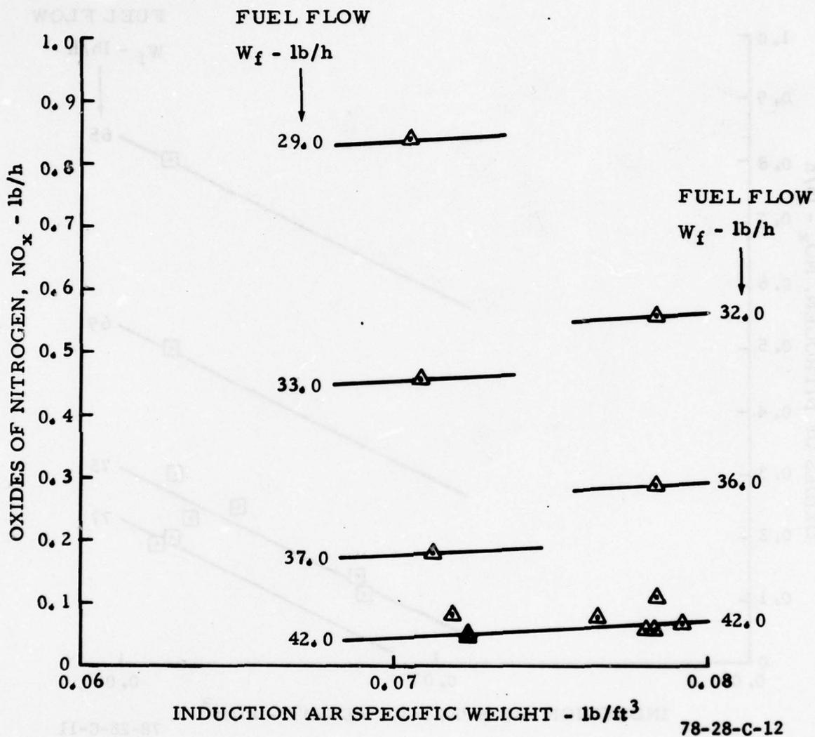
FIGURE C-12. OXIDES OF NITROGEN ( $NO_x$ ) AS A FUNCTION OF INDUCTION AIR SPECIFIC WEIGHT FOR SEVERAL APPROACH MODE CONSTANT FUEL FLOW SCHEDULES--AVCO LYCOMING IO-360-B1BD ENGINE
