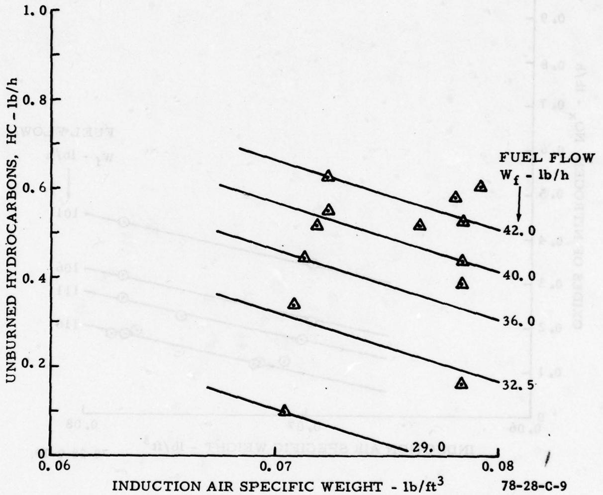
FIGURE C-9. UNBURNED EXHAUST HYDROCARBONS AS A FUNCTION OF INDUCTION AIR SPECIFIC WEIGHT FOR SEVERAL APPROACH MODE CONSTANT FUEL FLOW SCHEDULES—AVCO LYCOMING IO-360-B1BD ENGINE
