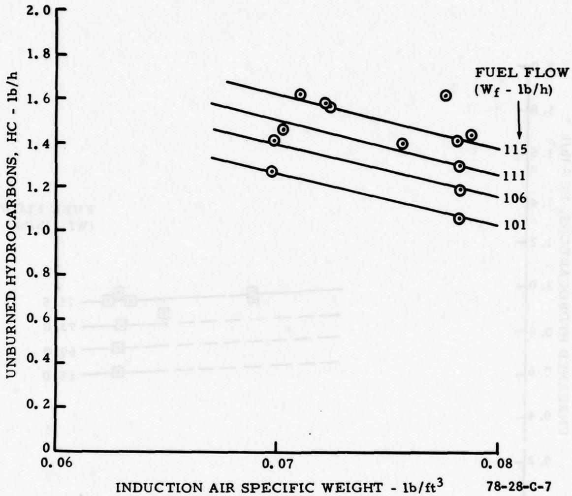
FIGURE C-7. UNBURNED EXHAUST HYDROCARBONS AS A FUNCTION OF INDUCTION AIR SPECIFIC WEIGHT FOR SEVERAL TAKEOFF CONSTANT FUEL FLOW SCHEDULES--AVCO LYCOMING IO-360-B1BD ENGINE
