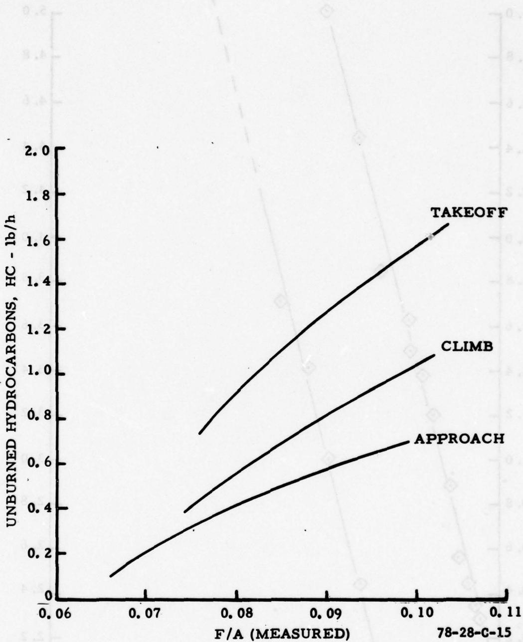
FIGURE C-17. SEA LEVEL HOT-DAY ( $T_1=103^\circ$  F) EMISSIONS CHARACTERISTICS FOR AN AVCO LYCOMING IO-360-B1BD ENGINE—UNBURNED HYDROCARBONS
