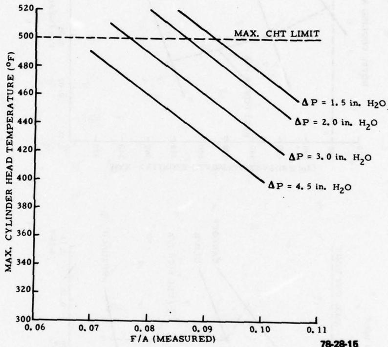
FIGURE 15. SEA LEVEL MAXIMUM CYLINDER HEAD TEMPERATURE VARIATIONS FOR DIFFERENT COOLING AIR DIFFERENTIAL PRESSURE CONDITIONS AND VARYING FUEL-AIR RATIOS--AVCO LYCOMING IO-360-B1BD ENGINE--TAKEOFF MODE
