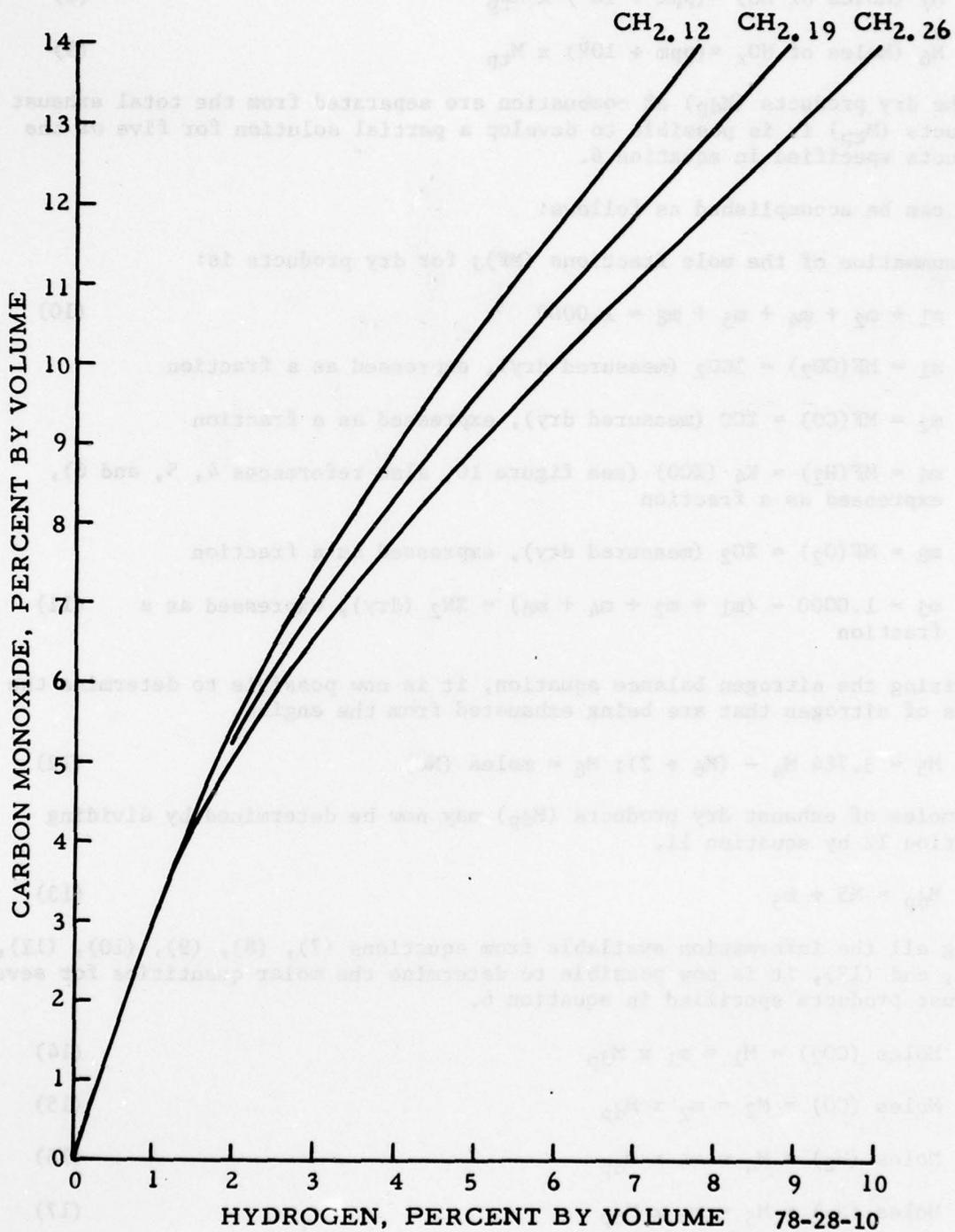
FIGURE 10. RELATION OF CARBON MONOXIDE AND HYDROGEN
