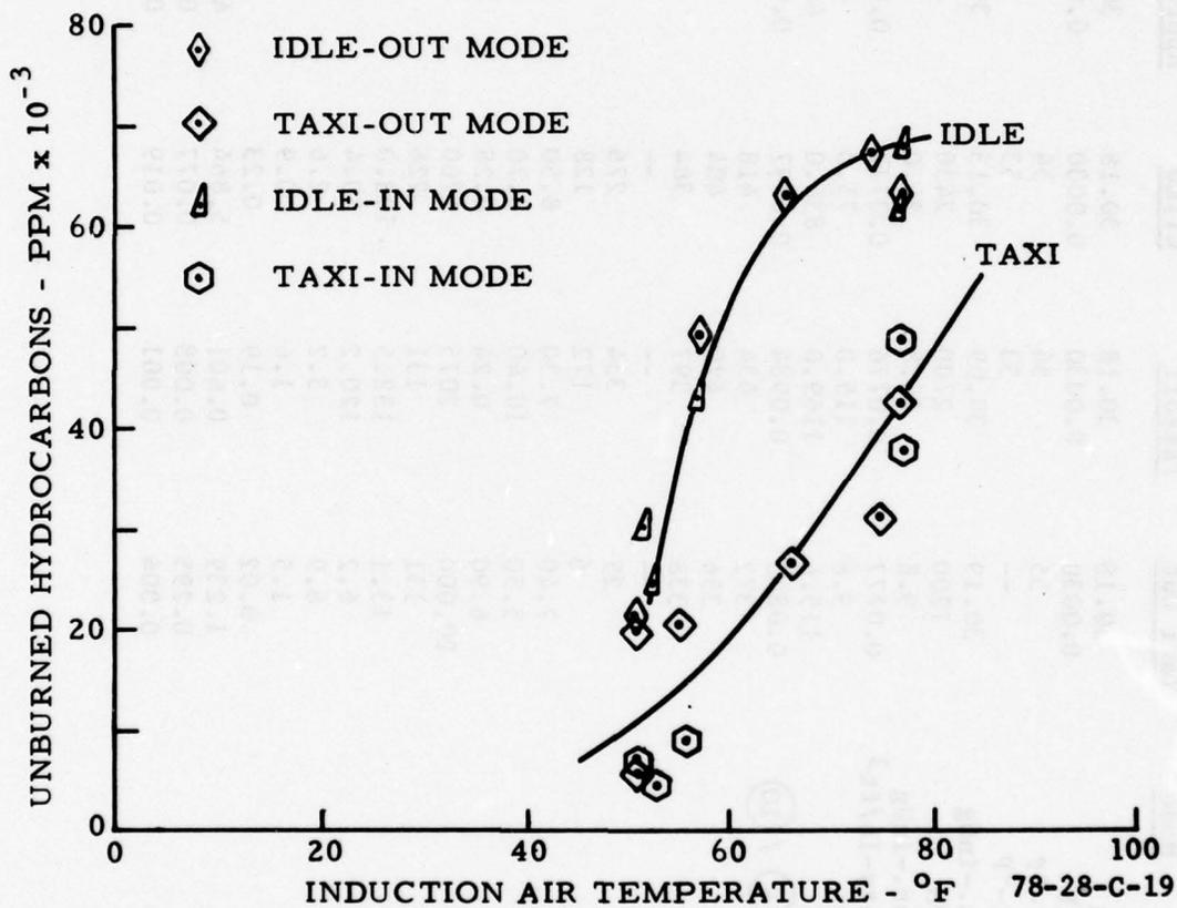
FIGURE C-19. EFFECTS OF INDUCTION AIR TEMPERATURE ON THE PRODUCTION OF EXHAUST UNBURNED HYDROCARBON EMISSIONS--AVCO LYCOMING IO-360-B1BD ENGINE
