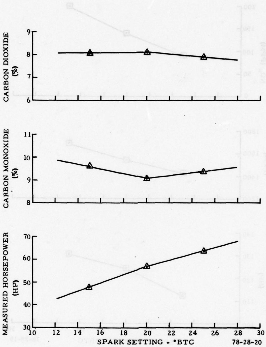
FIGURE 20. EFFECT OF VARYING SPARK SETTING ON ENGINE PERFORMANCE AND EXHAUST EMISSIONS—APPROACH MODE (CO<sub>2</sub> AND CO)
