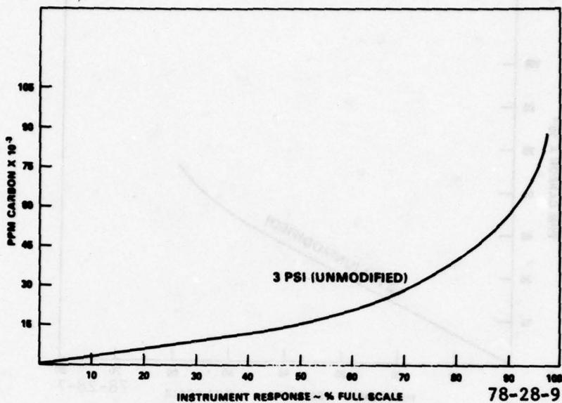
FIGURE 8. BECKMAN MODEL 402 THC ANALYZER (3 PSI UNMODIFIED)
