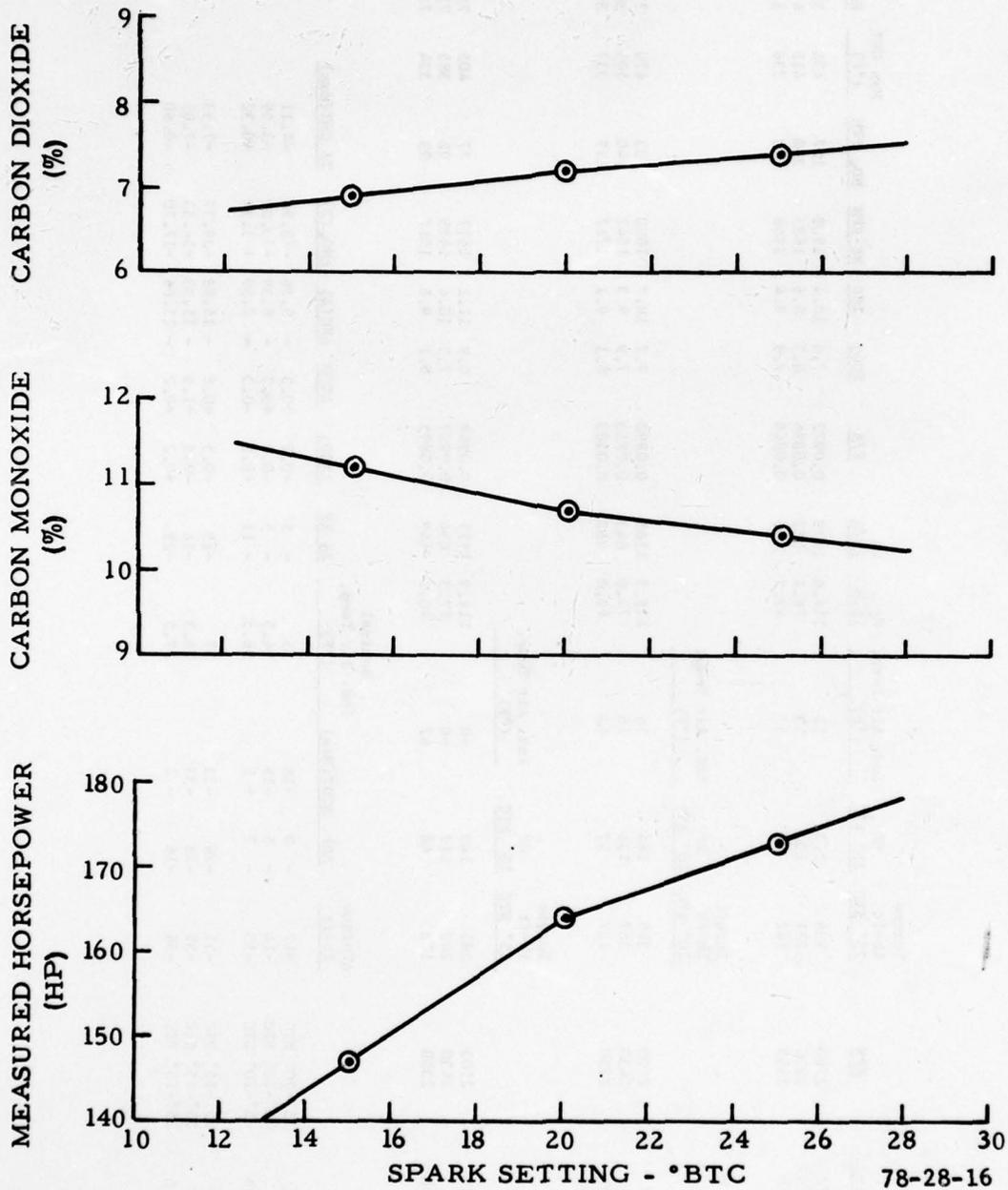
FIGURE 16. EFFECT OF VARYING SPARK SETTING ON ENGINE PERFORMANCE AND EXHAUST EMISSIONS--TAKEOFF MODE (CO<sub>2</sub> AND CO)
