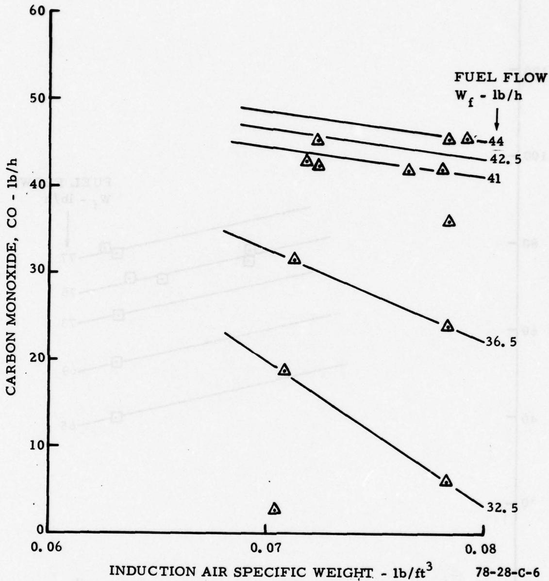
FIGURE C-6. EXHAUST CARBON MONOXIDE AS A FUNCTION OF INDUCTION AIR SPECIFIC WEIGHT FOR SEVERAL APPROACH MODE CONSTANT FUEL FLOW SCHEDULES--AVCO LYCOMING IO-360-B1BD ENGINE
