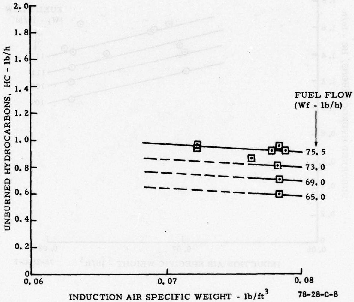
FIGURE C-8. UNBURNED EXHAUST HYDROCARBONS AS A FUNCTION OF INDUCTION AIR SPECIFIC WEIGHT FOR SEVERAL CLIMB MODE CONSTANT FUEL FLOW SCHEDULES--AVCO LYCOMING IO-360-B1BD ENGINE
