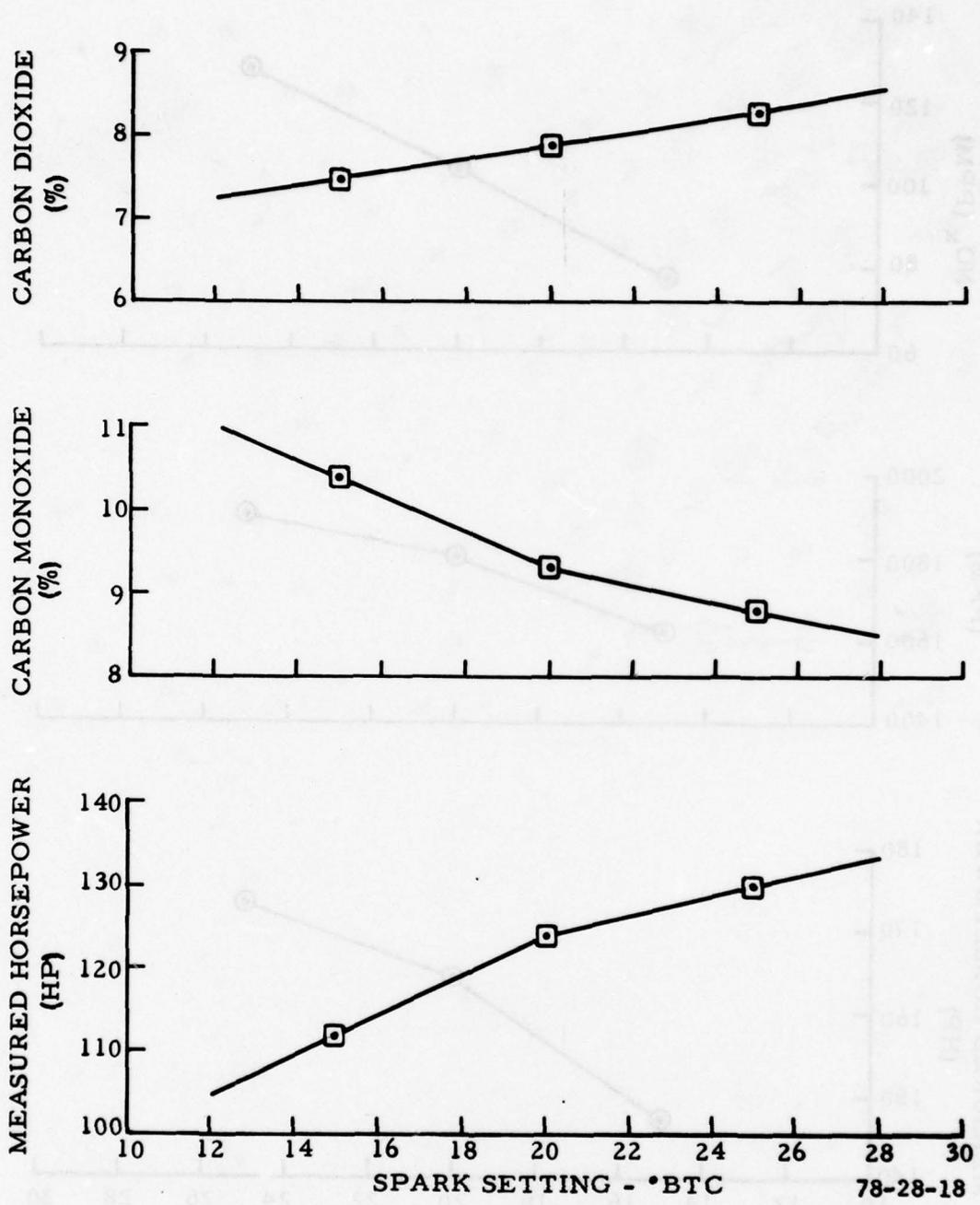
FIGURE 18. EFFECT OF VARYING SPARK SETTING ON ENGINE PERFORMANCE AND EXHAUST EMISSIONS—CLIMB MODE (CO<sub>2</sub> AND NO<sub>x</sub>)
