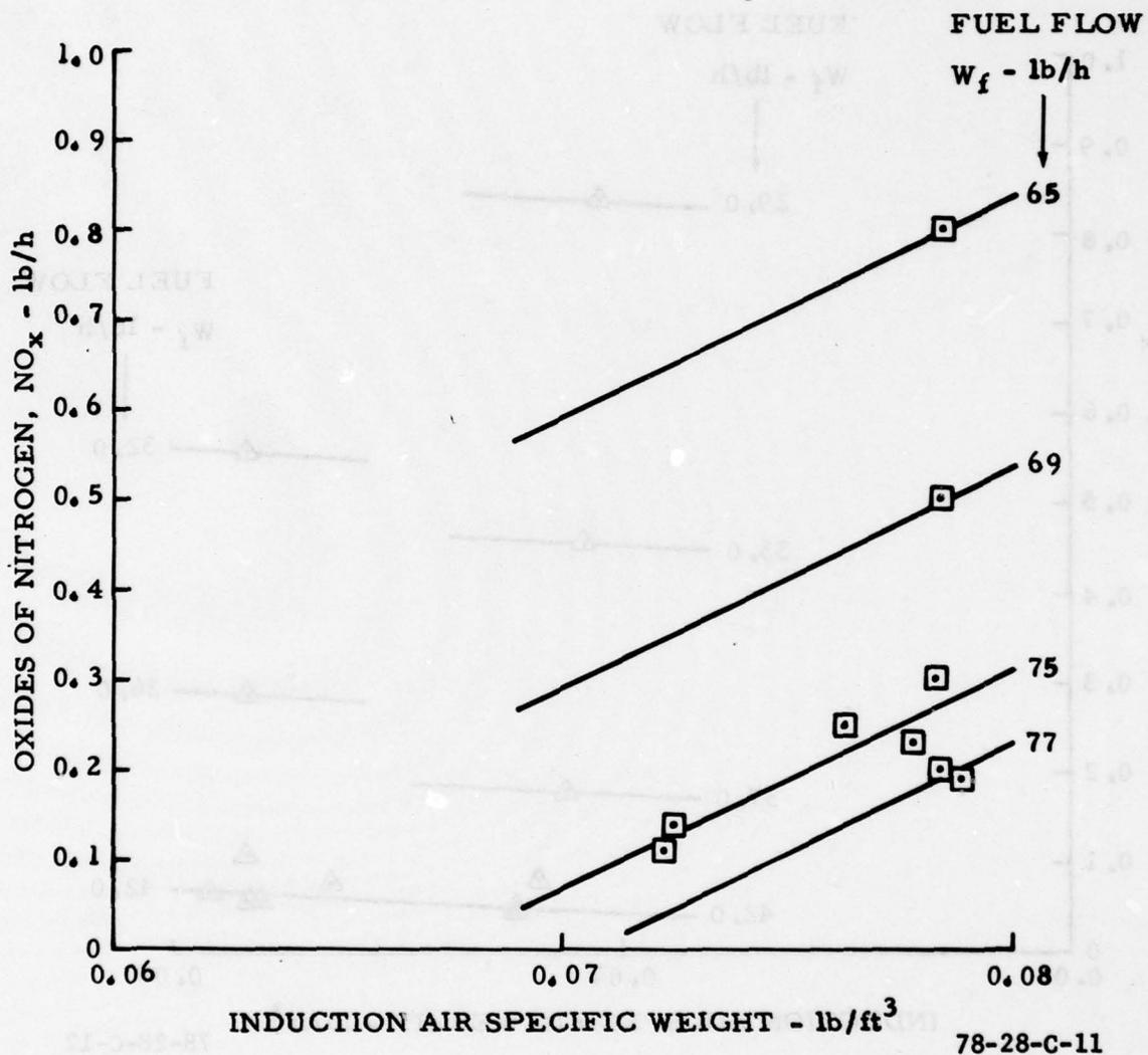
FIGURE C-11. OXIDES OF NITROGEN ( $NO_x$ ) AS A FUNCTION OF INDUCTION AIR SPECIFIC WEIGHT FOR SEVERAL CLIMB MODE CONSTANT FUEL FLOW SCHEDULES--AVCO LYCOMING IO-360-B1BD ENGINE
