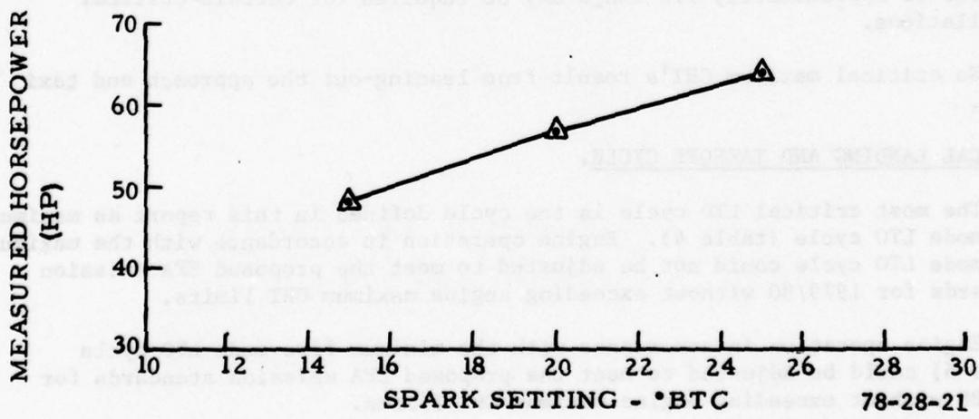
FIGURE 21. EFFECT OF VARYING SPARK SETTING ON ENGINE PERFORMANCE AND EXHAUST EMISSIONS--APPROACH MODE (HC AND NO<sub>x</sub>)
