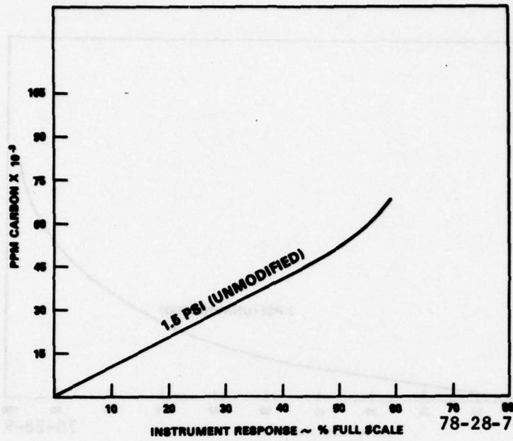
FIGURE 6. BECKMAN MODEL 402 THC ANALYZER (1.5 PSI UNMODIFIED)
