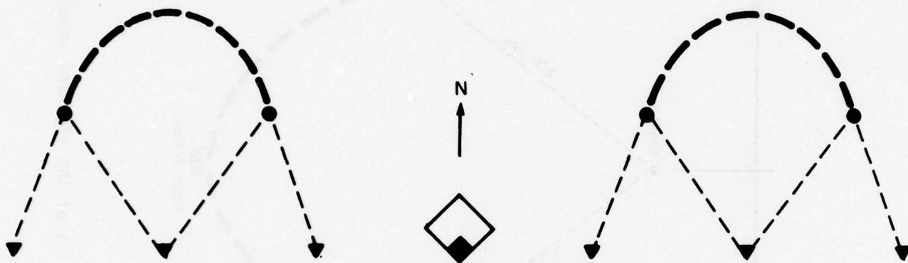
Figure 14. The standard mooring arrangement, re-oriented to take better advantage of the southerly winds
