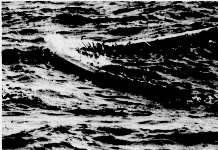
Figure 50. An example of splashover, which occurred with all three booms that remained afloat and undamaged.
