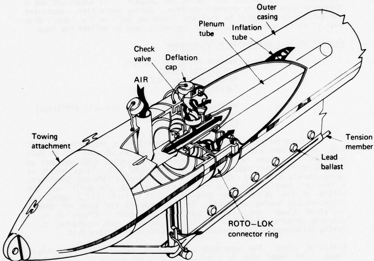
Figure 6. The Bennett Towing Attachment and the Offshore Boom
