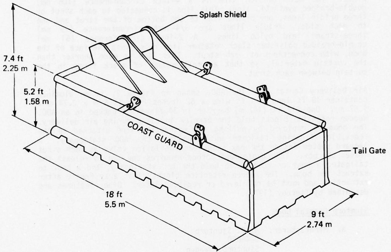
Figure 2. Sketch of the USCG Air Delivery Container
