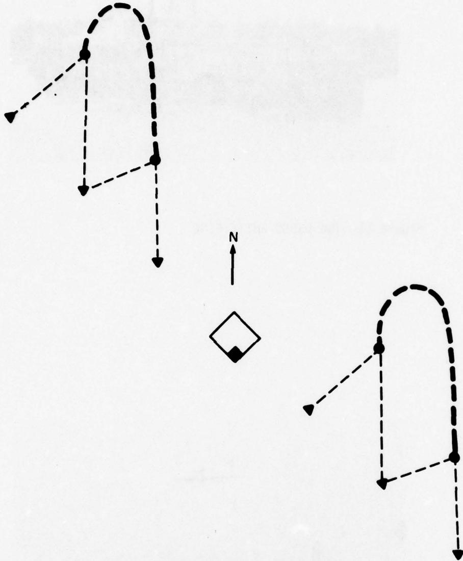
Figure 13. The initial mooring arrangement, showing the shapes the booms typically assumed due to the predominantly southern winds
