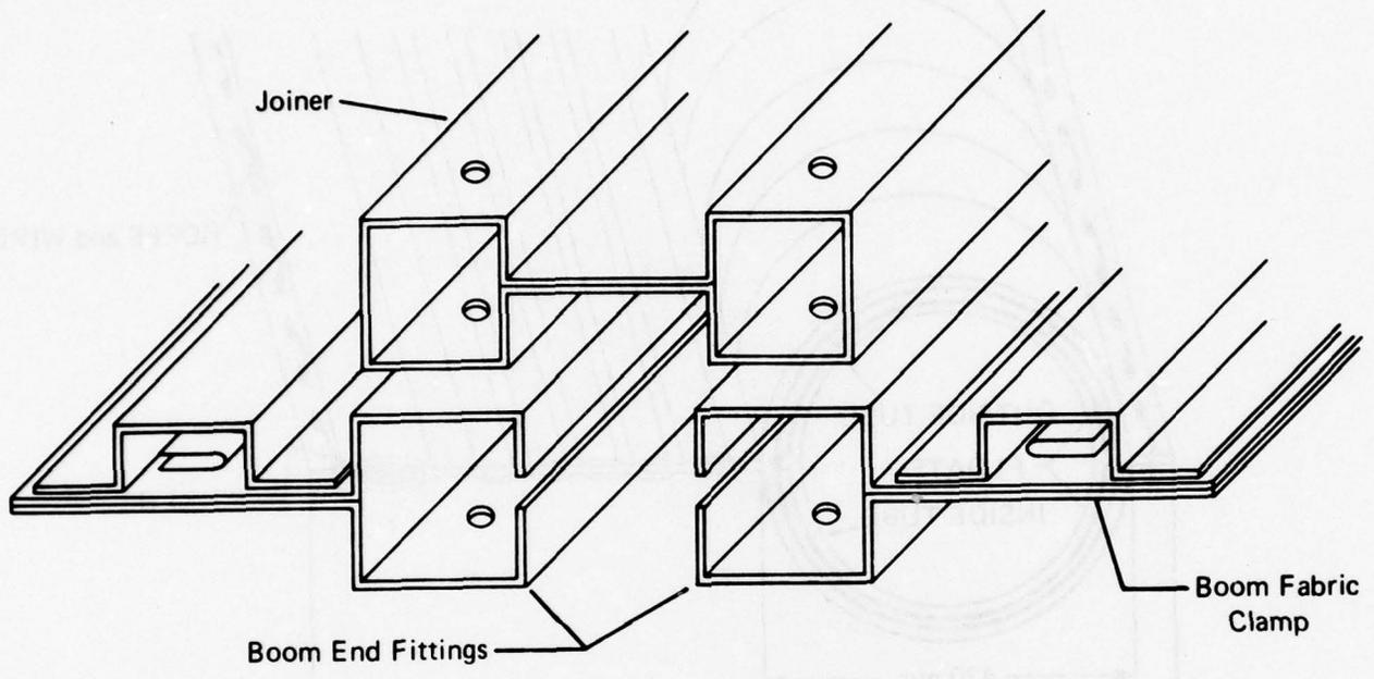
Figure 4. The Sjuntorp Boom Connectors
