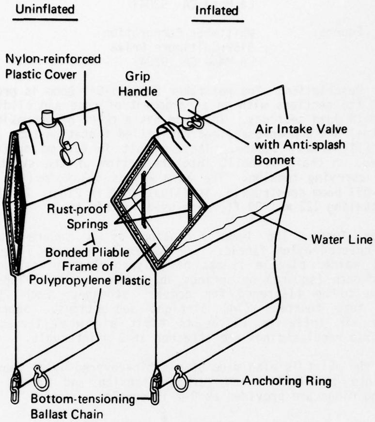
Figure 7. The Whittaker Expandi-Oil Boom
