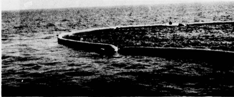
Figure 44. Crewmen in a Zodiac boat tending the Bennett boom, which is sinking at the connectors. A video target may be seen to the left of the Zodiac boat.
