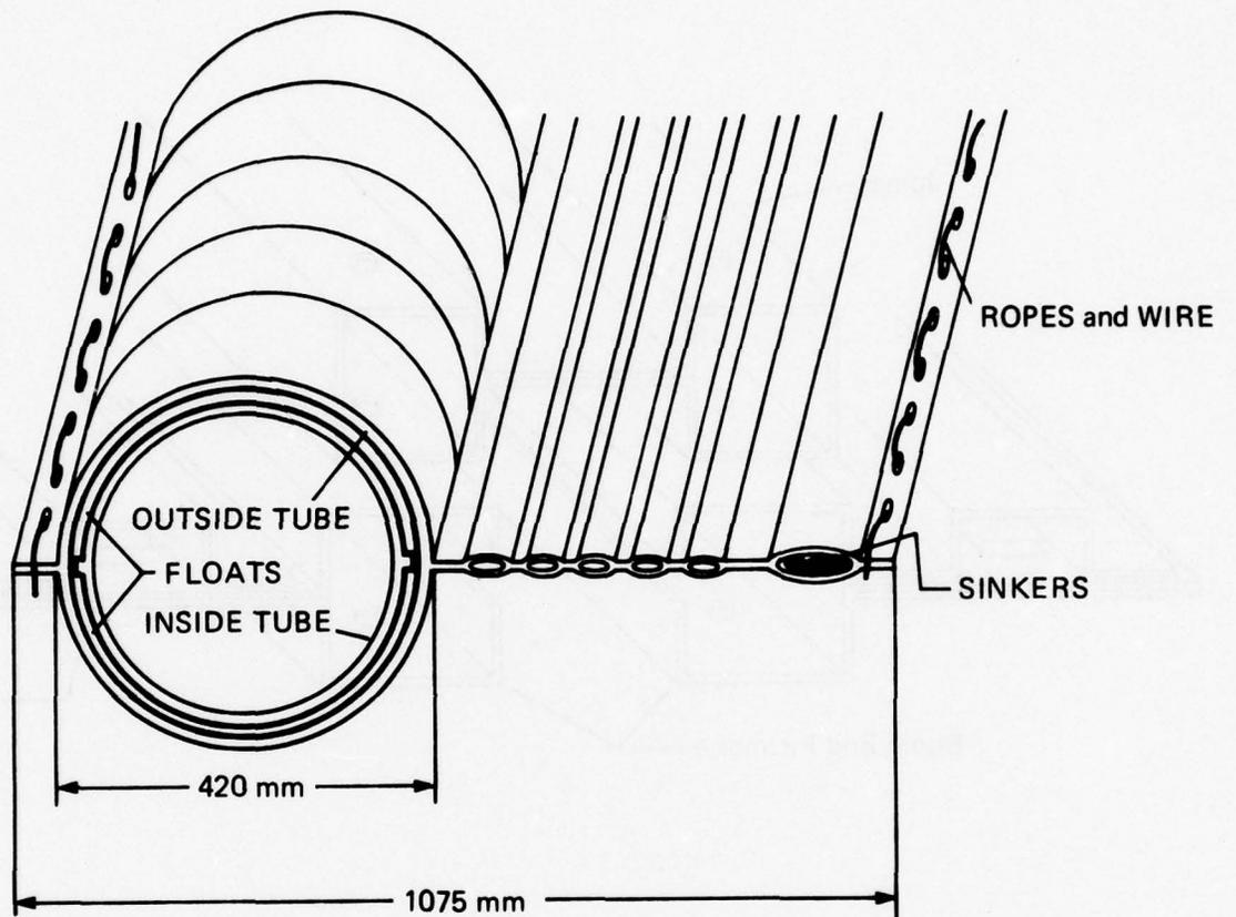
Figure 3. Sketch of the Sjuntorp Coastal Boom
