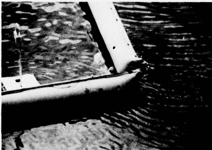
Figure 30. Close-up showing the skirt of Sjuntorp boom rising to the surface.
