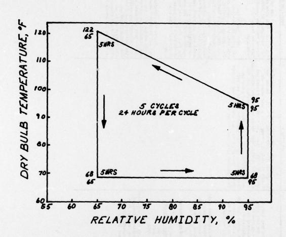
Figure 1 - TELCAM Temperature/Relative Humidity Test
