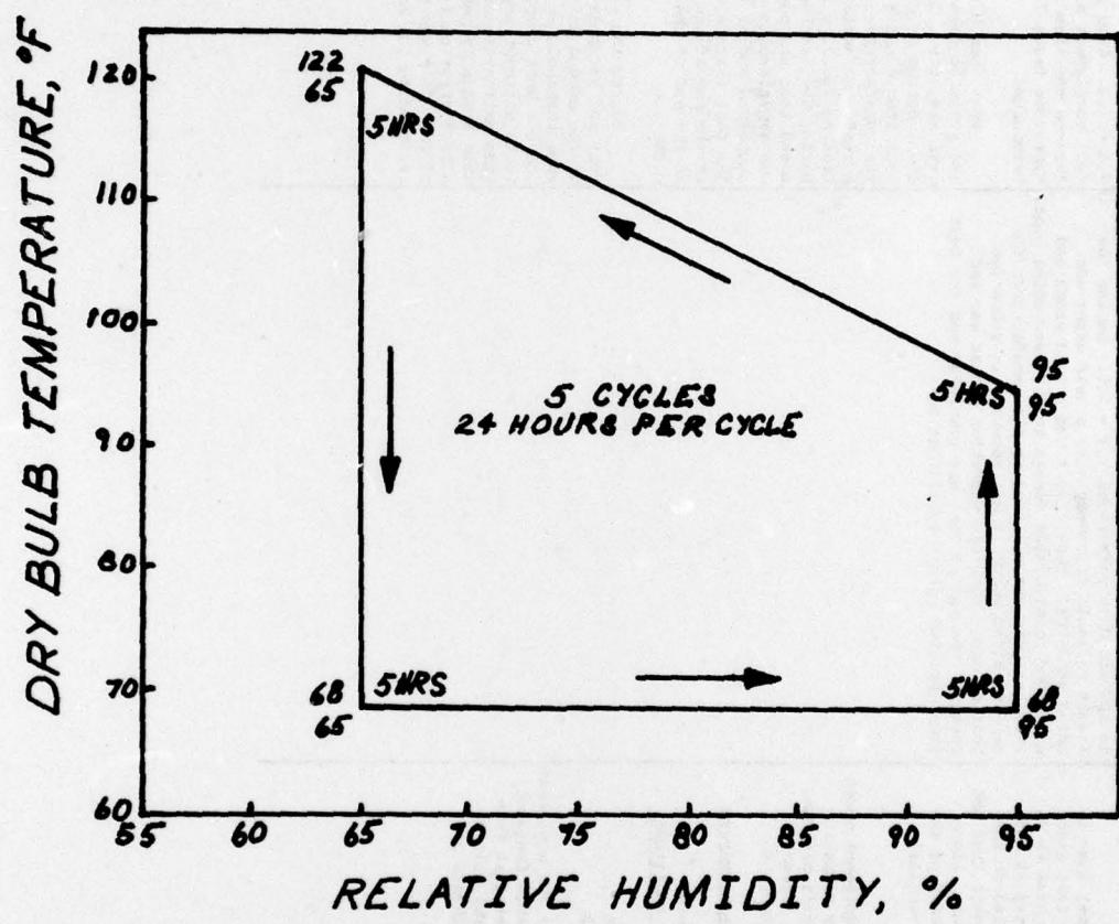
Figure 1 - TELCAM Temperature/Relative Humidity Test
