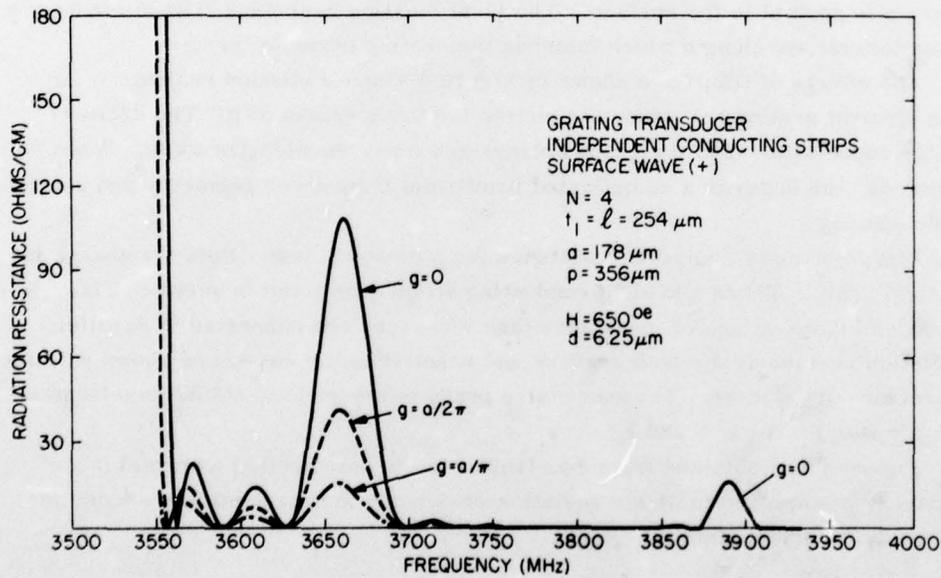
Figure 4. Radiation Resistance as a Function of Liftoff
