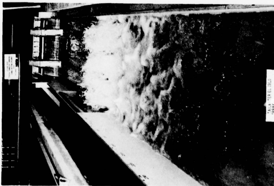
Photo 3. Flow conditions in Spillway A stilling basin; unit discharge 67.7 cfs/ft, pool el 224.1, gate opening 4 ft (sheet 1 of 2)
