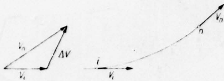
Figure 11. Change in the vector of velocity \Delta \vec{V} between velocity \vec{V}_n and the velocity at a current instant.
