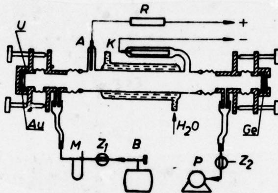
Fig. 1. Structural scheme of CO<sub>2</sub> flow laser: A - anode, K - cathode, Au - gold mirror, Ge - germanium mirror, U - seals, P - rotary pump, B - cylinder, M - oil pressure gauge, Z<sub>1</sub> and Z<sub>2</sub> - valves.
