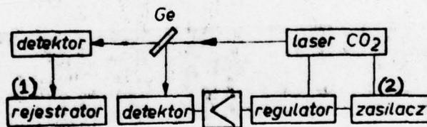
Fig. 7. Block diagram of system for stabilizing CO<sub>2</sub> laser output power
