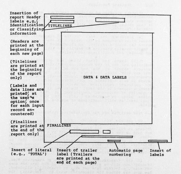
Figure 3. Printed Output
