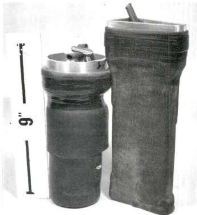
(a) Tooling for trapezoidal billets
