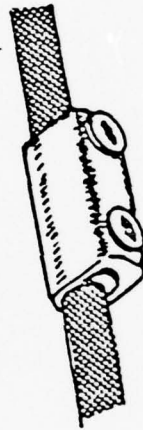
2-Hole Screw-Type Terminal
