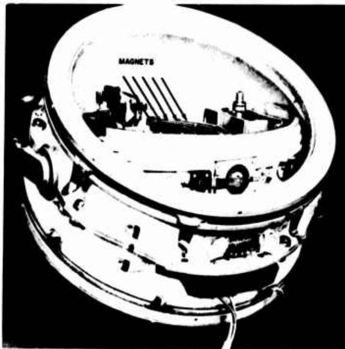
Figure 44.—Early German magnetic mine firing device.
