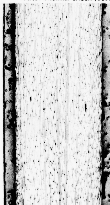
Figure 37: Aluminum Clad Laminate After Heat Aging (50X)
