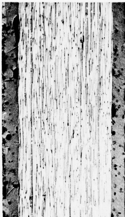
Figure 34: Aluminum Clad Laminate Before Thermal Shock (50X)
