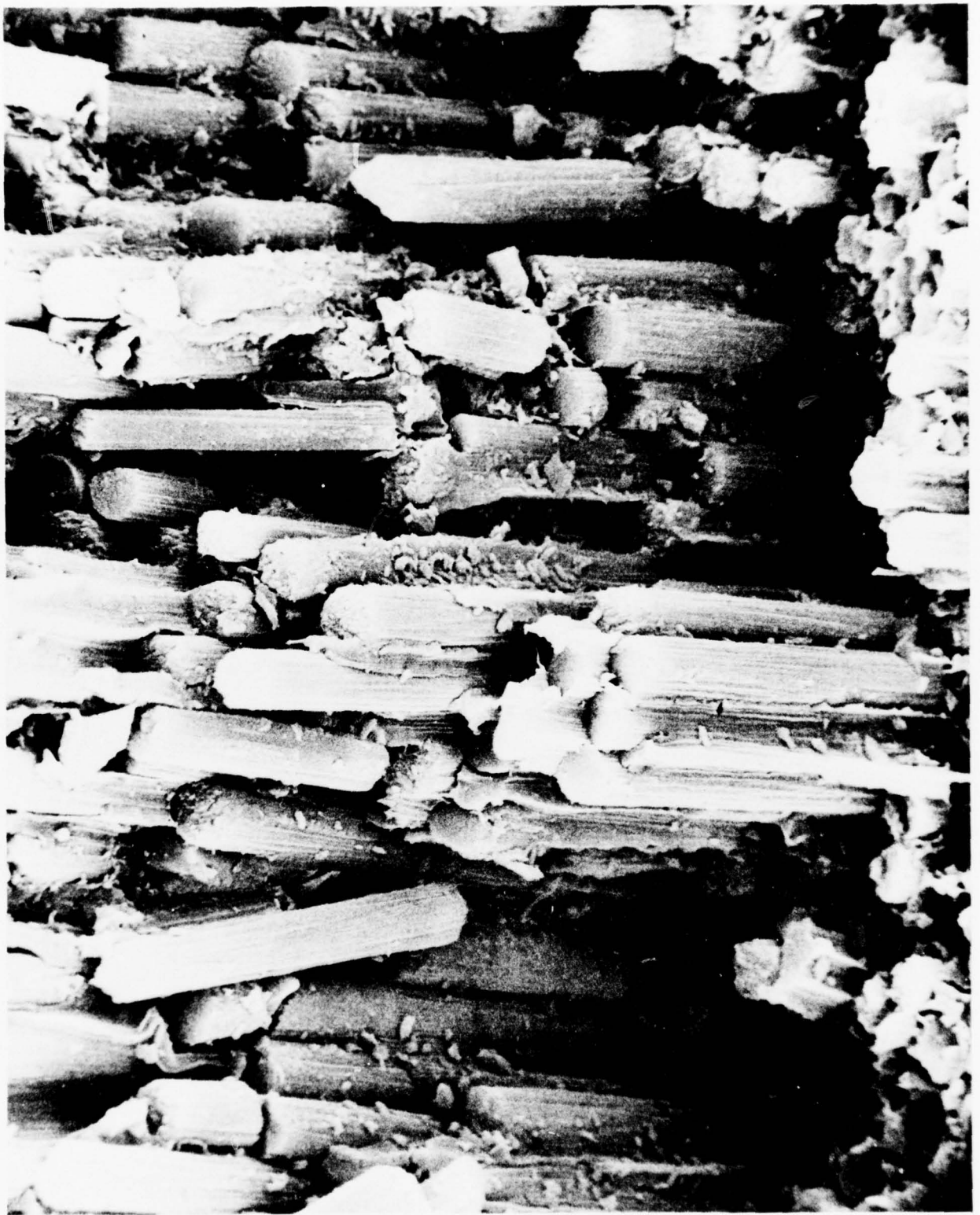
Figure 4: PKXA .41/HM-S Unidirectional Graphite Composite (600X)
