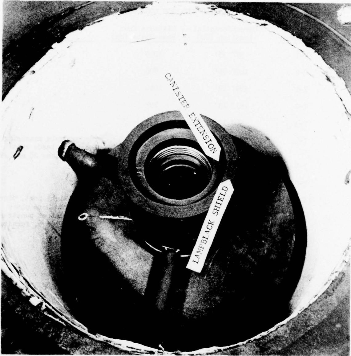
Fig. A-13. Furnace assembly to the lampblack shield level.
