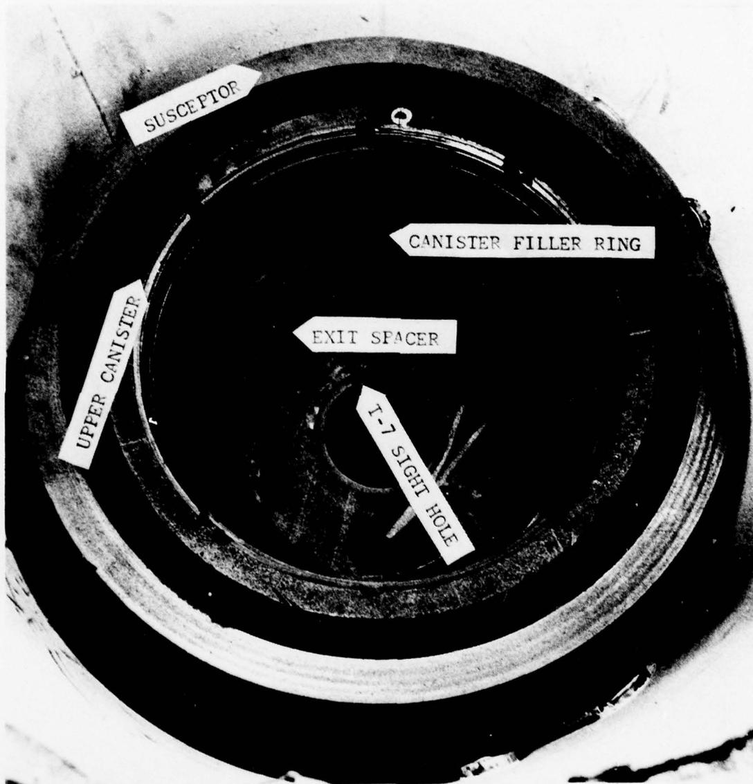
Fig. A-10. Furnace assembly to the upper canister level.
