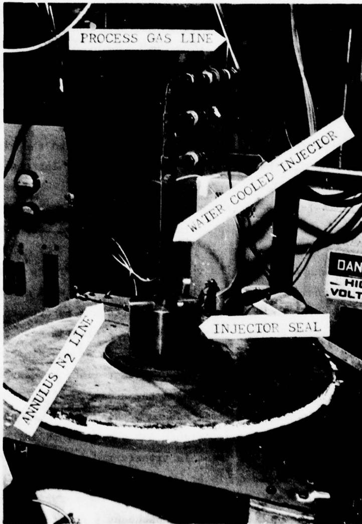
Fig. A-4. Furnace top details.
