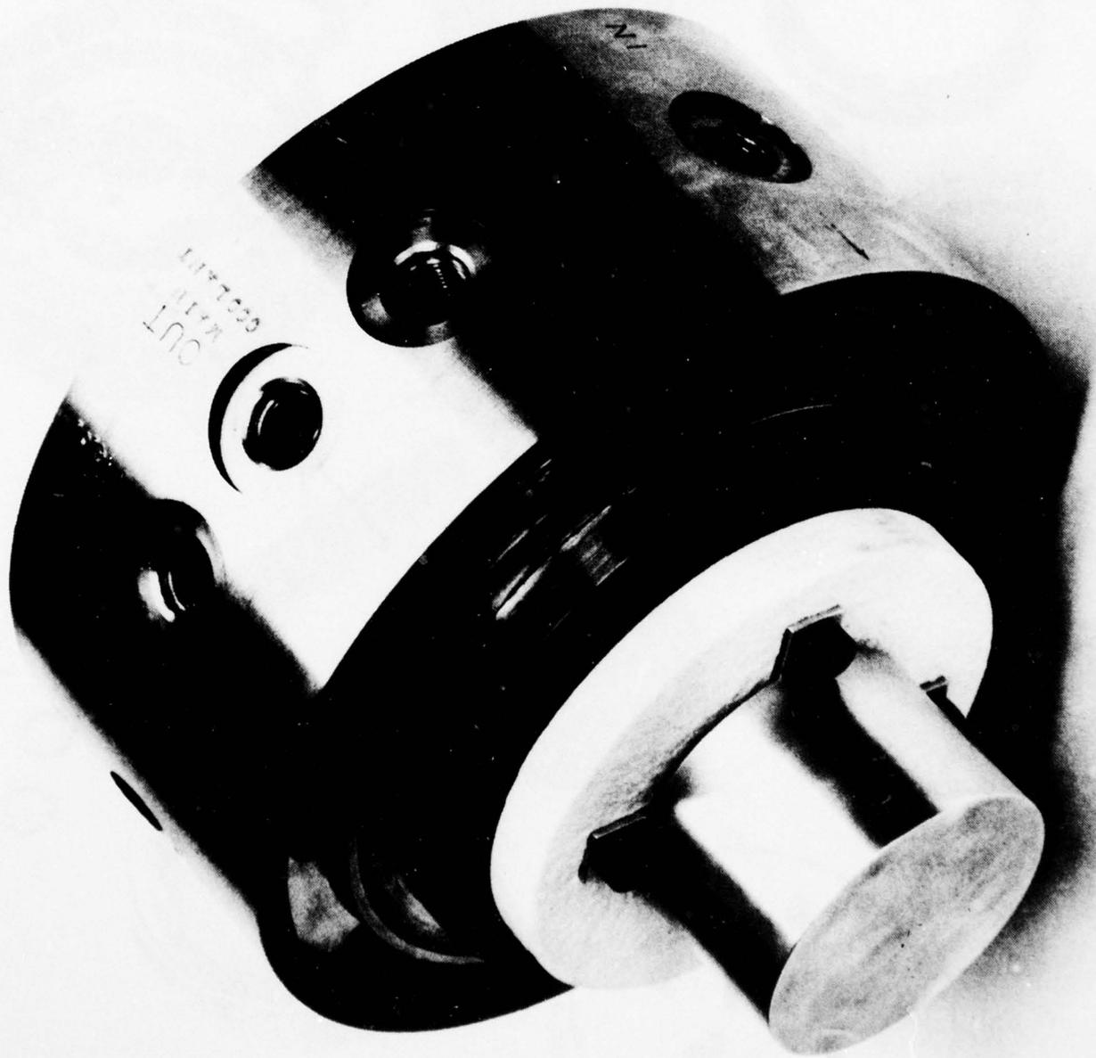
Figure 39. Rotary Seal Test Fixture
