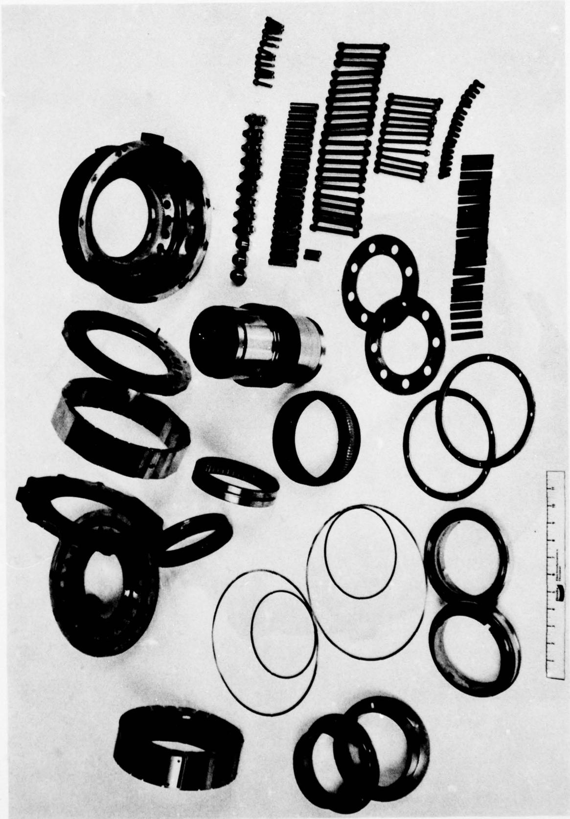
Figure 2. Prototype Actuator Model HL-043-U1 Components
