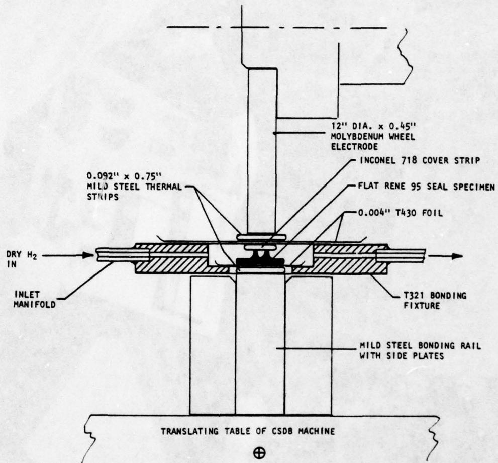
Figure 26. Cross Section of Bonding Lay-Up For CSDB of Flat Seal Teeth Bars.
