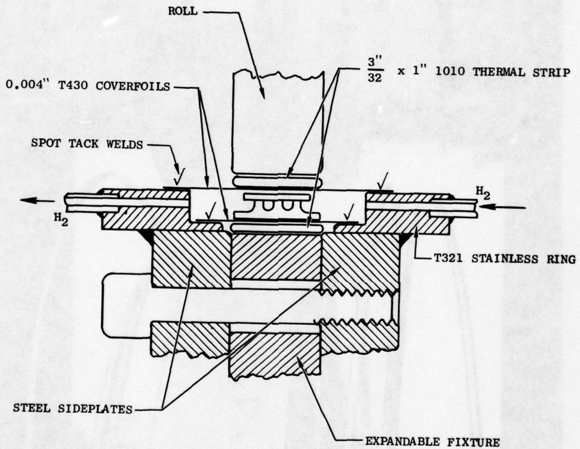
Figure 9. Cross-Section of Bonding Lay-Up For CSDB of Seal Teeth Rings.
