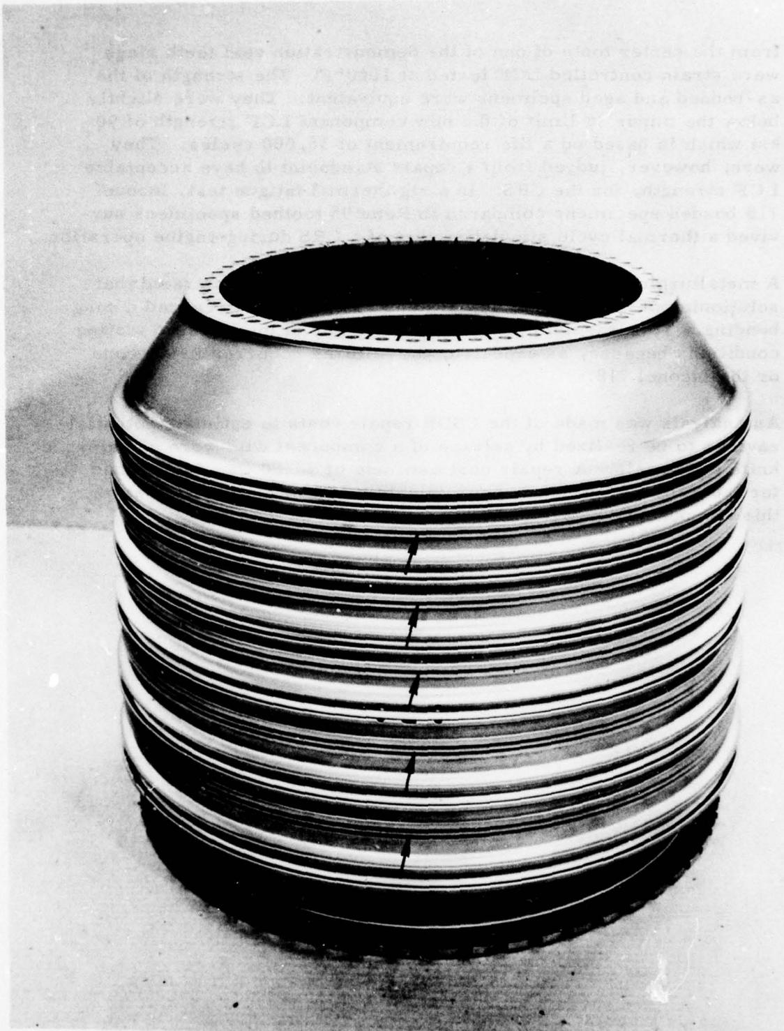
Figure 2. F101 René 95 Compressor Rotor Spool Stages 4 Through 9.
