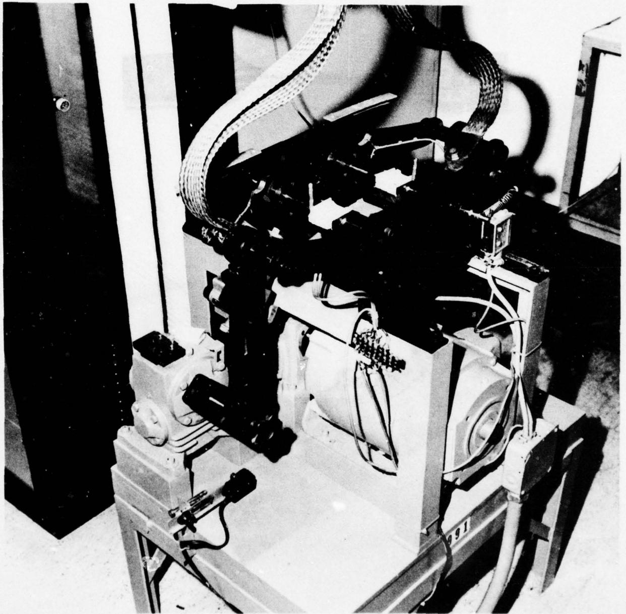
Figure 44. Forreast Four Point Bending LCF Machine.
