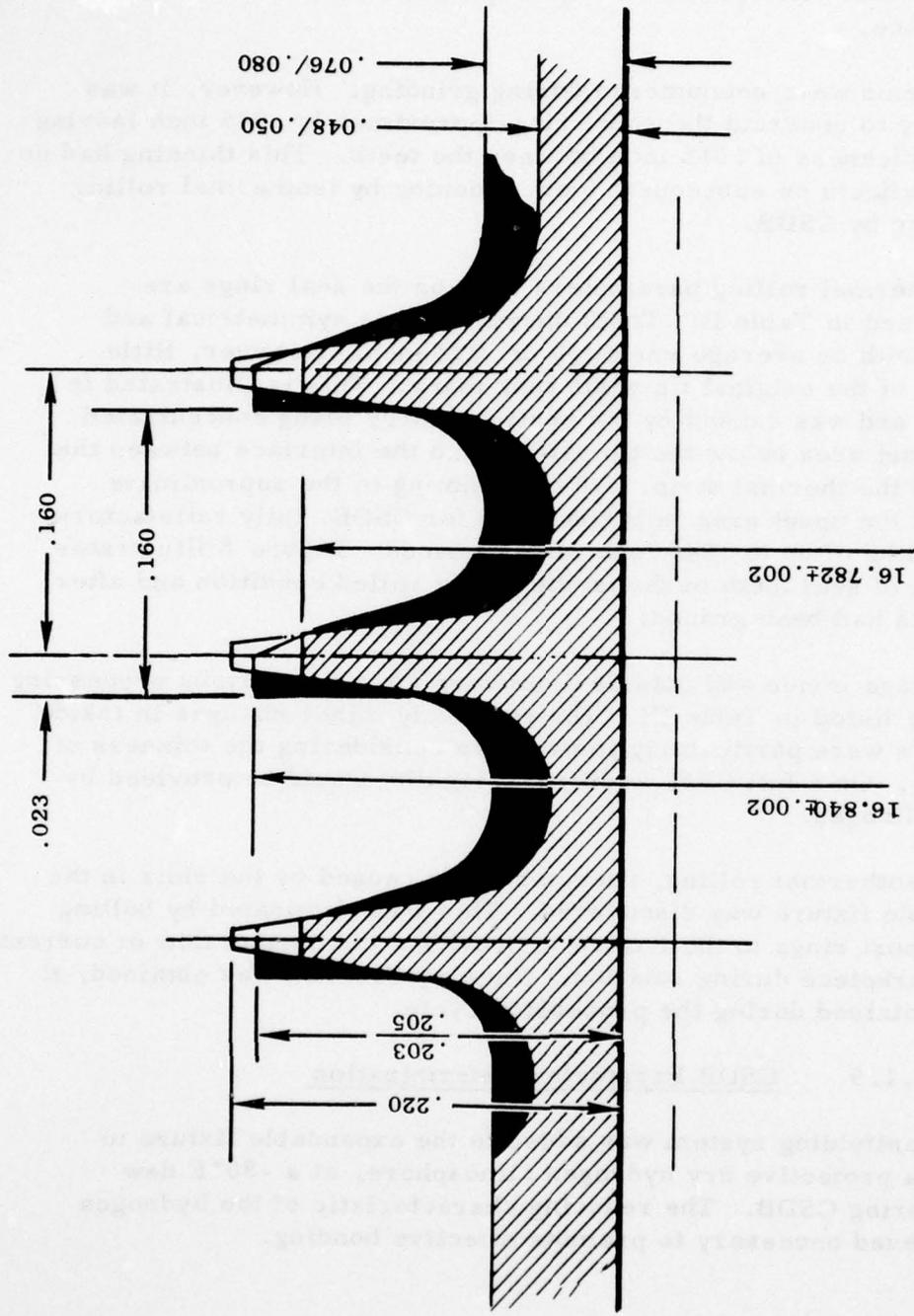
Figure 6 Remachined Seal Teeth Profiles
