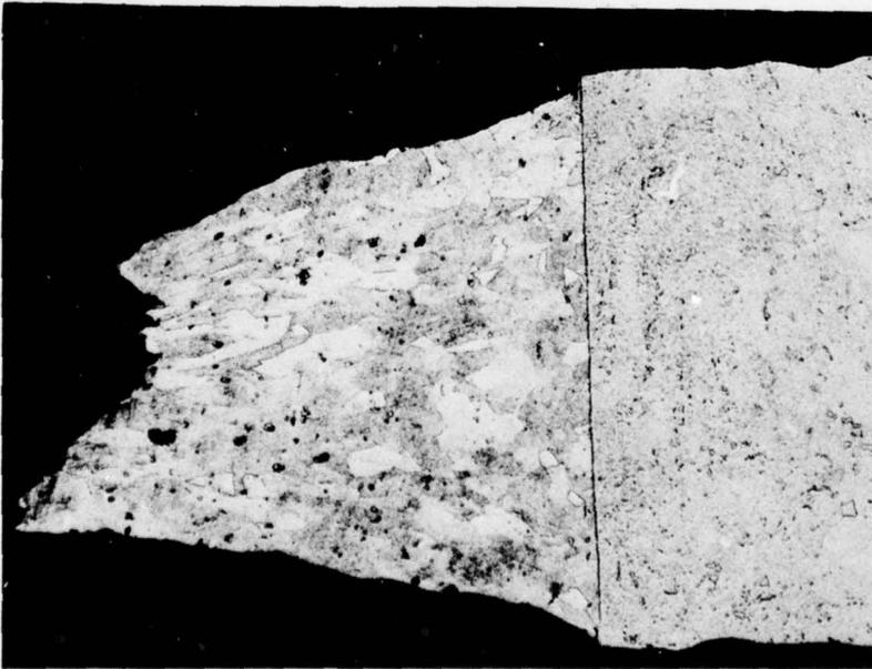
Figure 36. Room Temperature Failures in As-Bonded Tensile Specimen.
