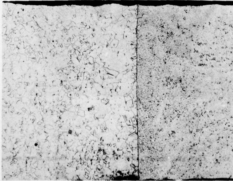
Figure 37. Bond Areas of Stress Rupture Specimen #9.
