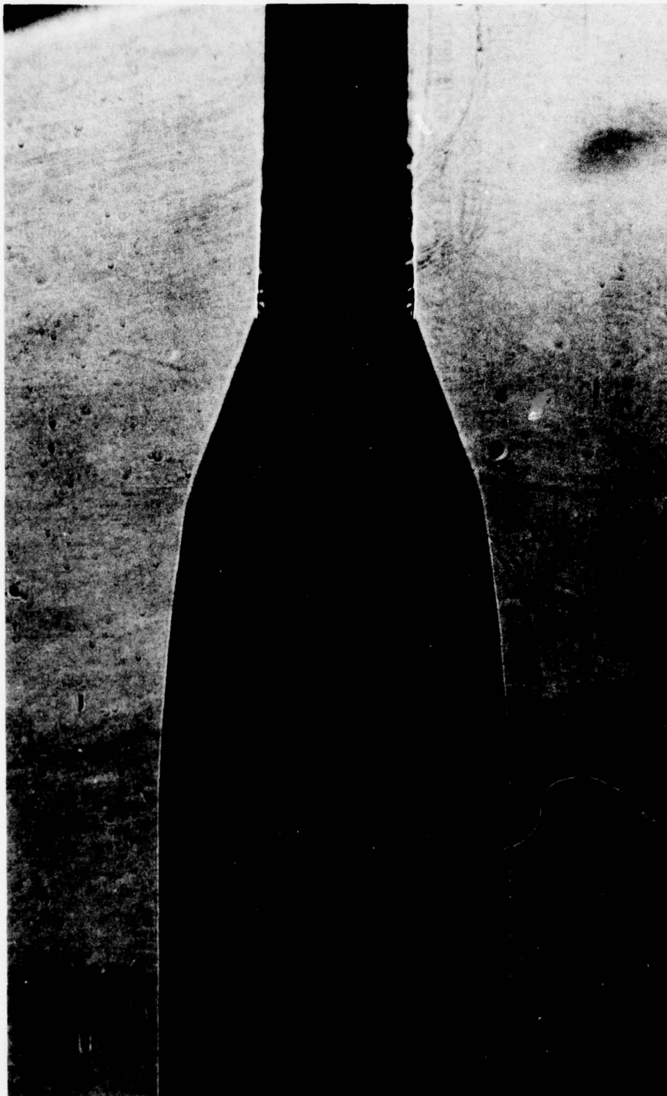
Figure 23. Cruise Nozzle; Annular Sting Plume Contour Schlieren, M_{\infty} = 0.6
