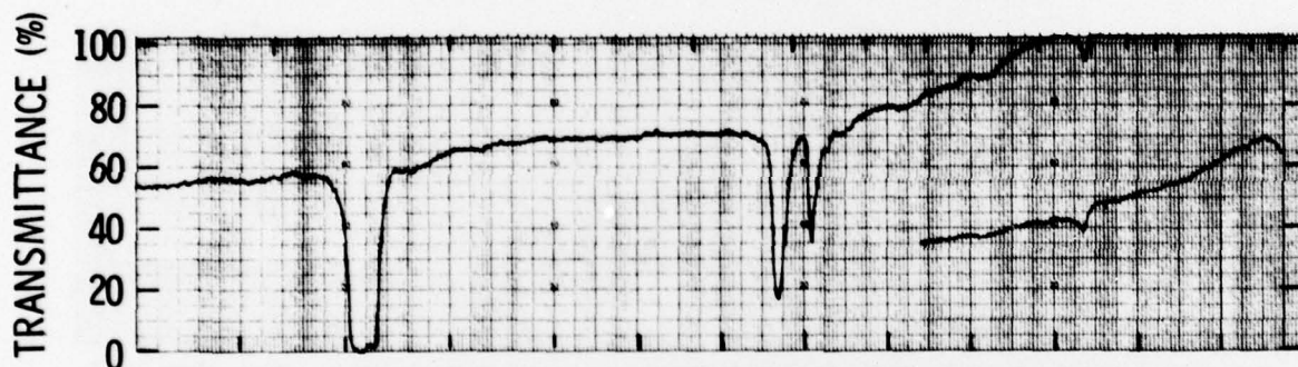
Fig. 32. Infrared Spectrum of 2% Lead Naphthenate in Apiezon C After Heating at 200°C for One Hour (KBr)
