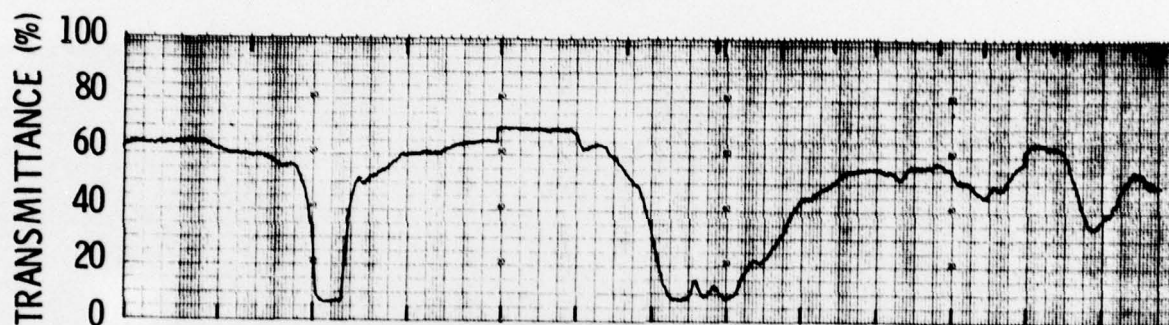
Fig. 20. Infrared Spectrum of Lead Naphthenate on Surface of KBr Pellet
