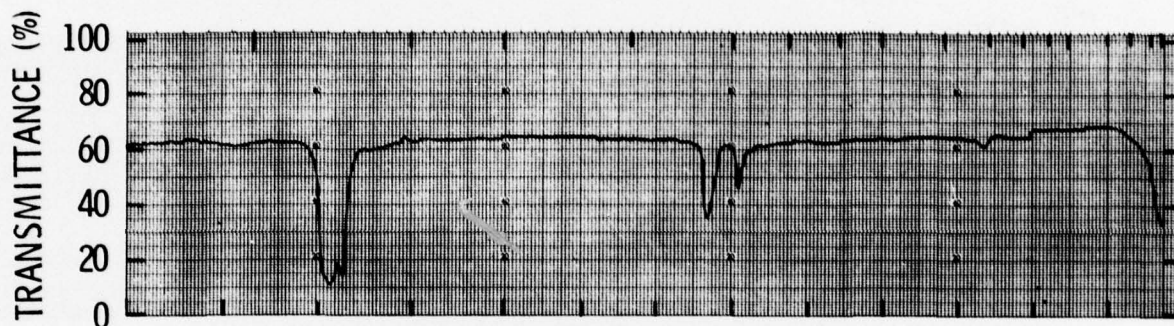
Fig. 17. Infrared Spectrum of 2% Lead Naphthenate in Apiezon C (KBr)
