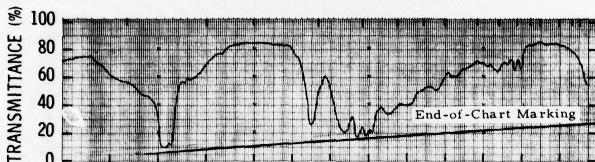
Fig. 29. Infrared Spectrum of Oil Layer Resulting from Reaction of Lead Naphthenate + 10% H 2 SO 4 . Mixture Heated at 100°C for 10 min (KRS-5)
