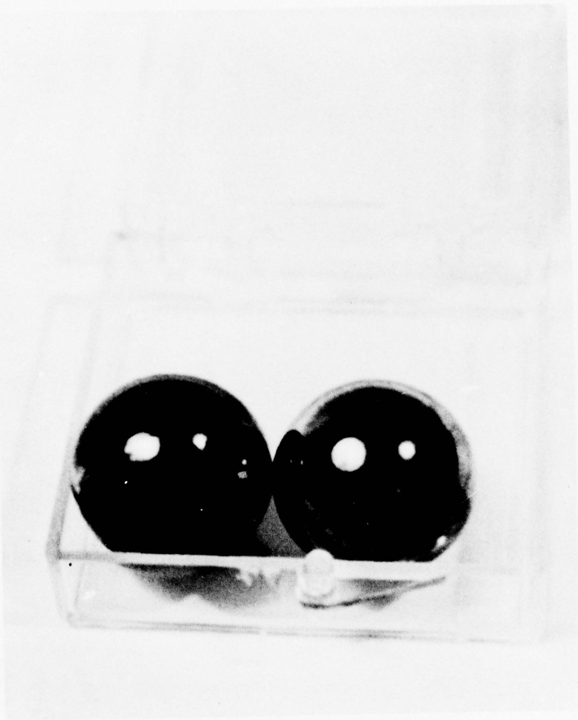
Fig. 1 - Balls from bearing 6B: left ball, as received; right ball, after deposit removal by NaOH
