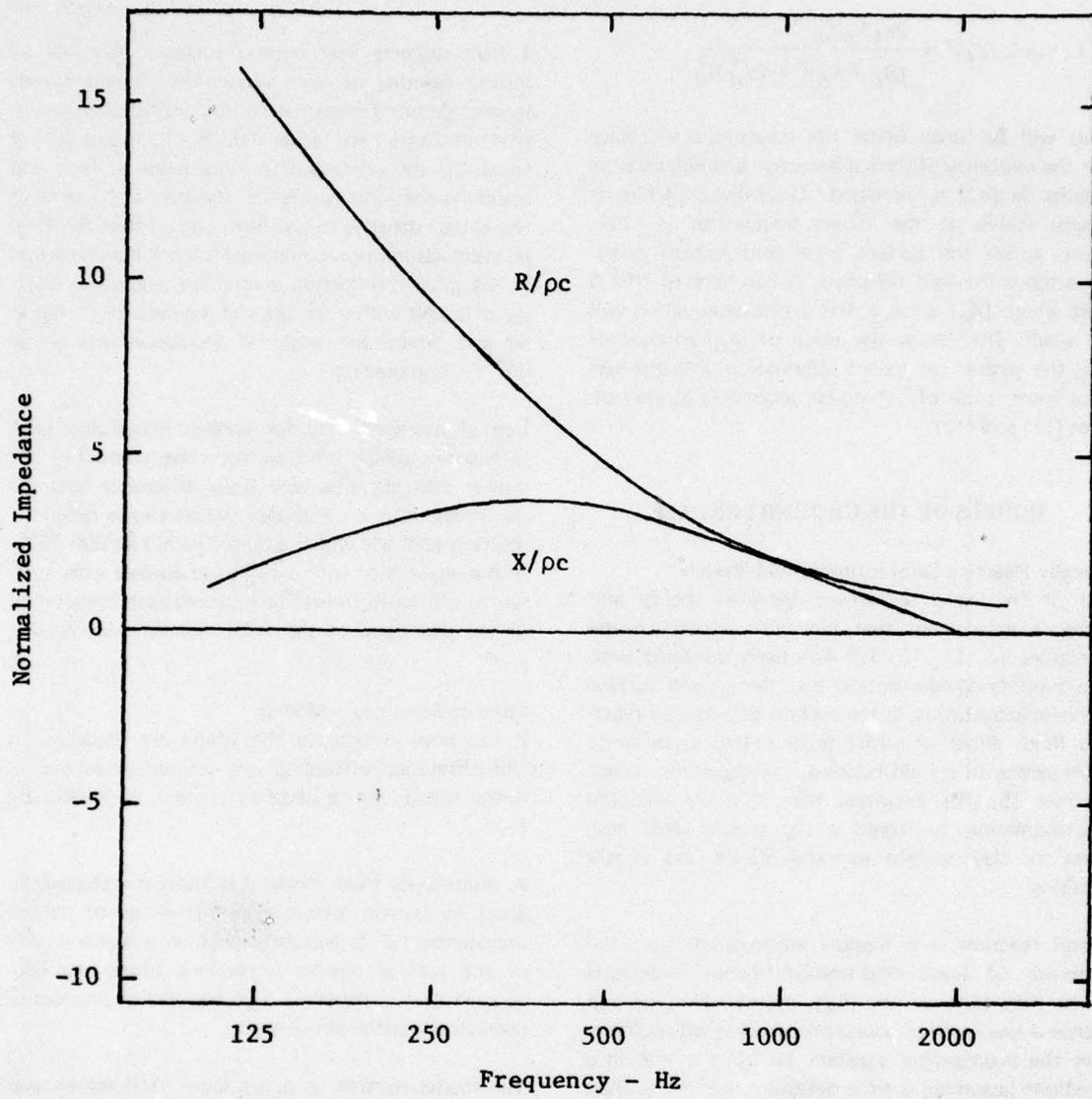
Figure 3. Normalized Impedance Data for Ground Showing Positive Imaginary Part (PSU)
