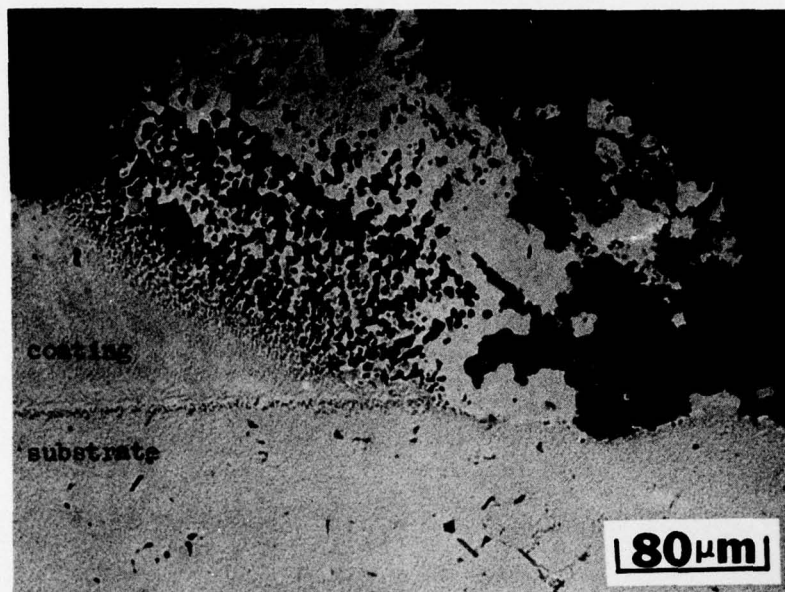
Figure 31a. Sidewise consumption of PWA 68 emanating from massive edge failure.
